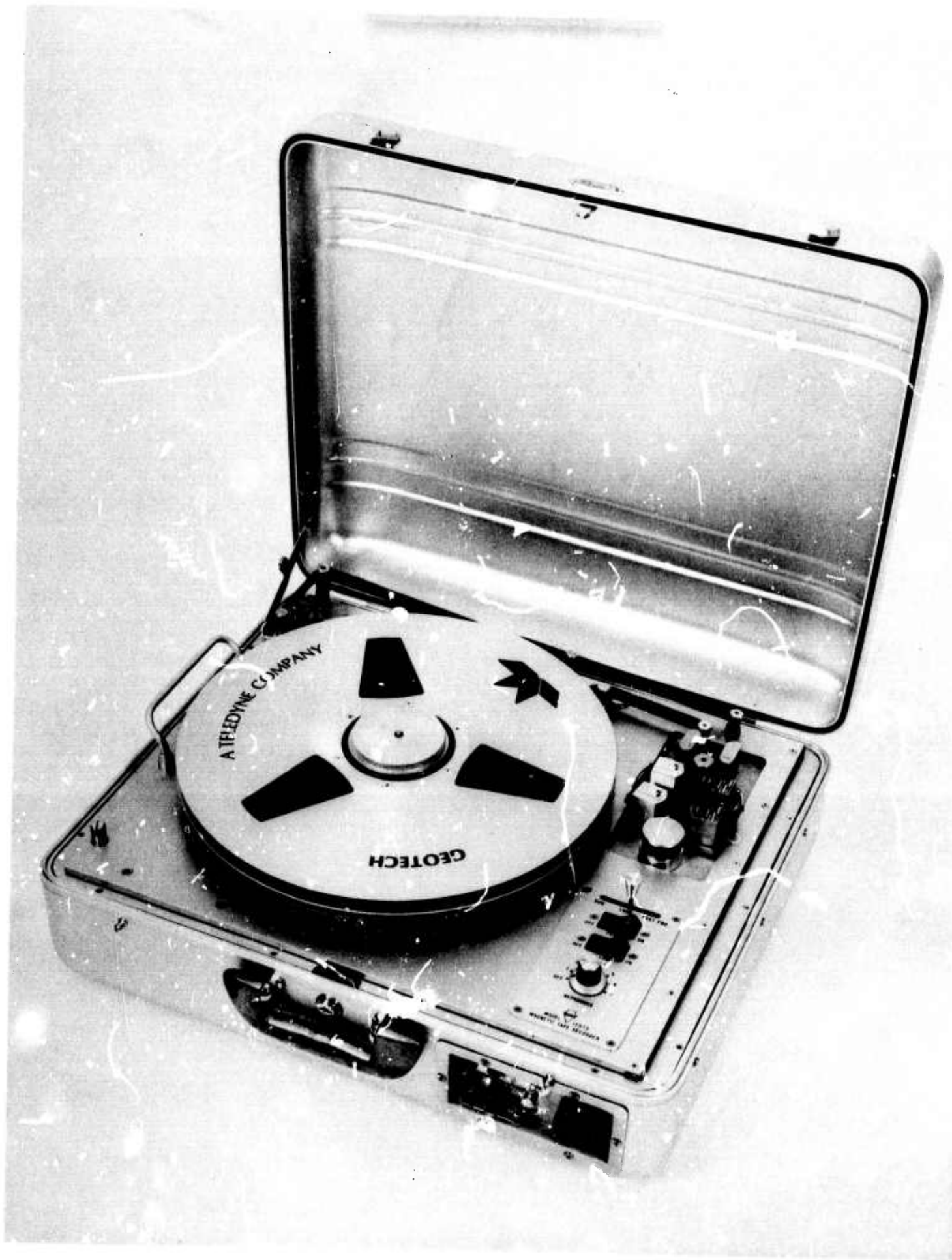
Figure 29. Photograph of Geotech Model 17373 magnetic tape recorder
