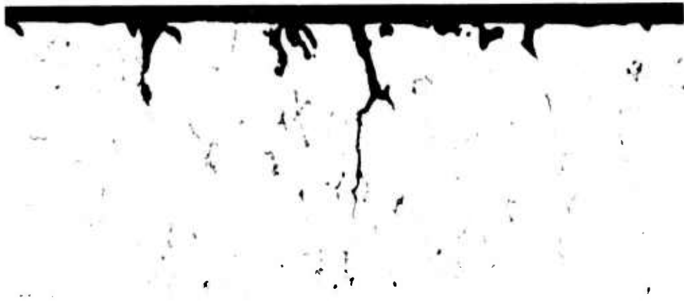
SPECIMEN 6B T6 12.5 DAYS TO FAILURE
