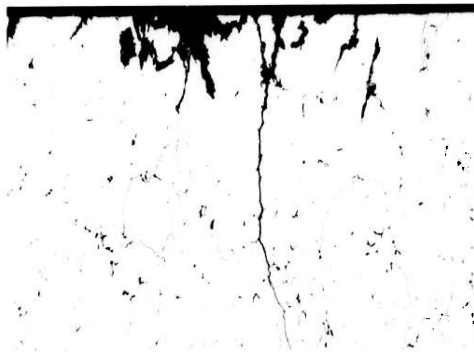
Figure 43. Cross Sections of Stress-Corrosion Specimens Tested in Tension at 35 KSI. Specimen Blanks Were Quenched in 140°F Water. Keller's Etch (100X).
