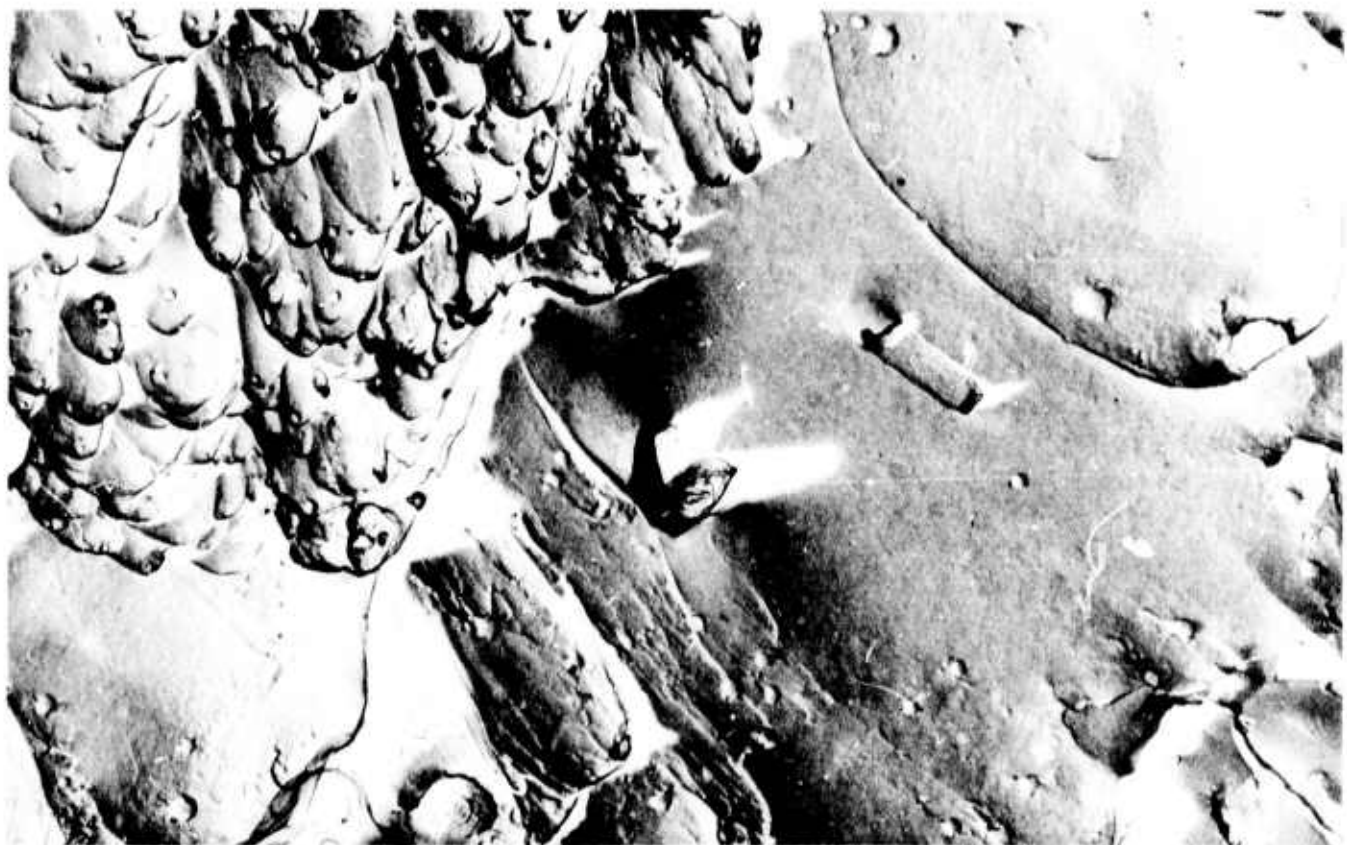
Figure 17. Typical Electron Fractographs of Tension Specimen 59 (Shown in Figure 12). Fracture Features on This Specimen Showed Small and Large Transgranular Dimples (A and B), Intergranular Dimples (C), and Intergranular Fracture (D) (6100X).
