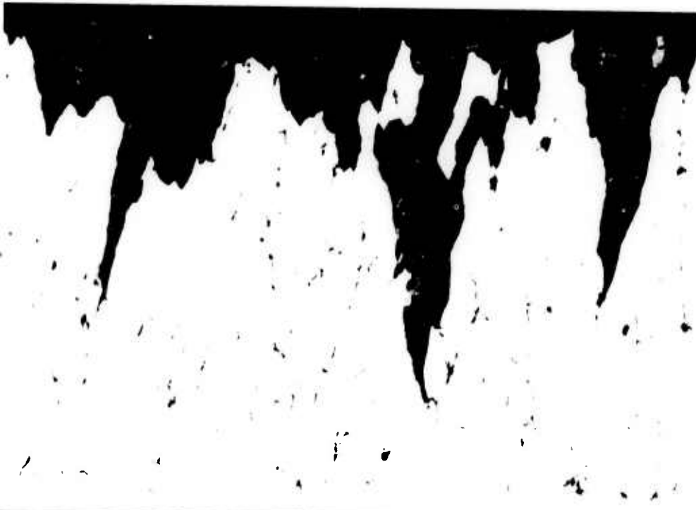
SPECIMEN 12A T6 + 30 HR AT 325°F REMOVED UNFAILED AFTER 90 DAYS
