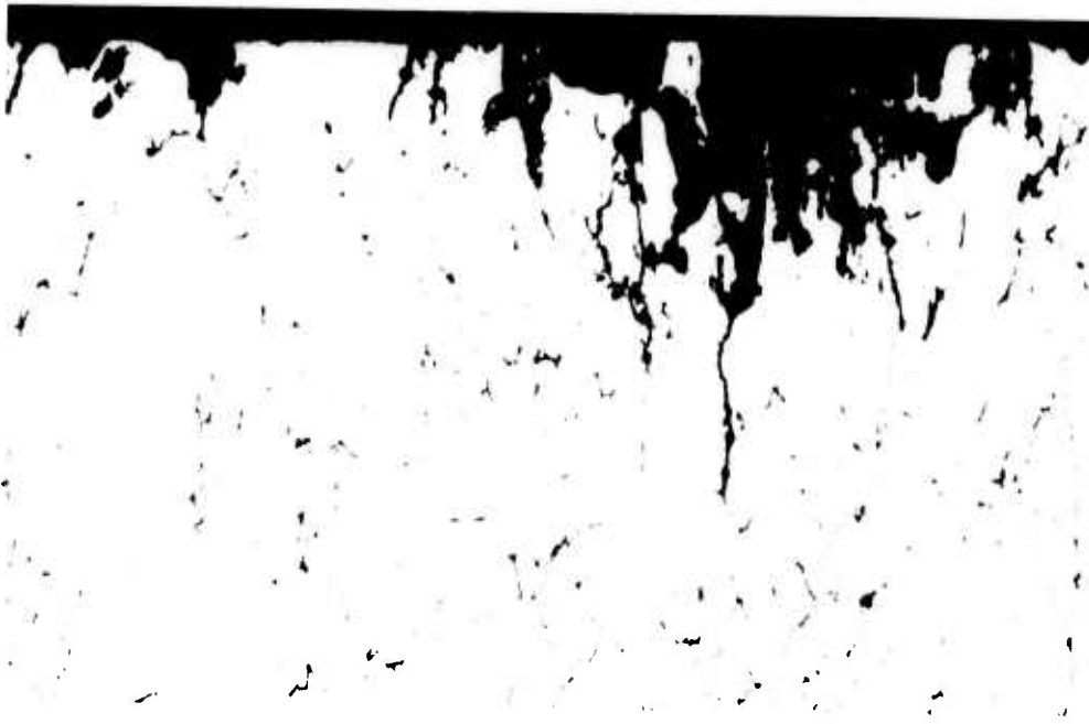
SPECIMEN 10C T6 + 20 HR AT 325°F REMOVED UNFAILED AFTER 90 DAYS
