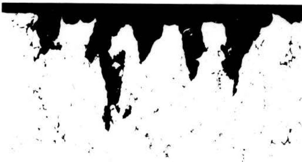
SPECIMEN 20B T6 + 50 HR AT 325° F REMOVED UNFAILED AFTER 90 DAYS
