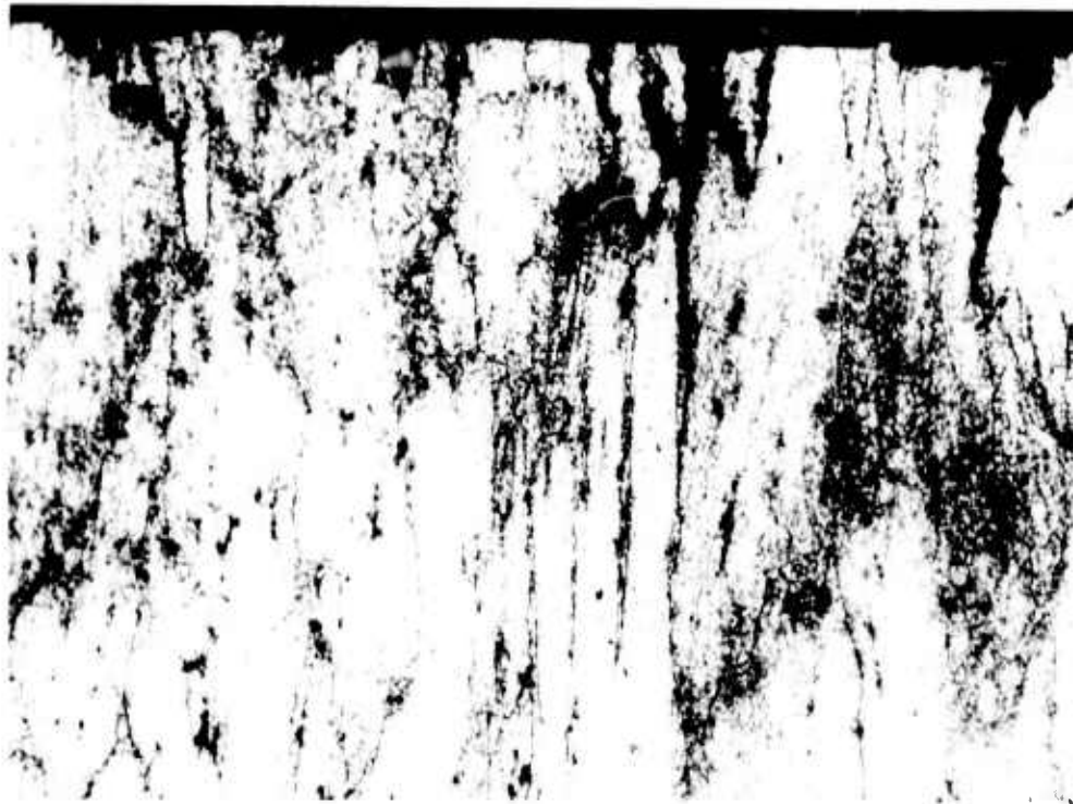
SPECIMEN 36C T6 + 20 HR AT 325°F 76 DAYS TO FAILURE
