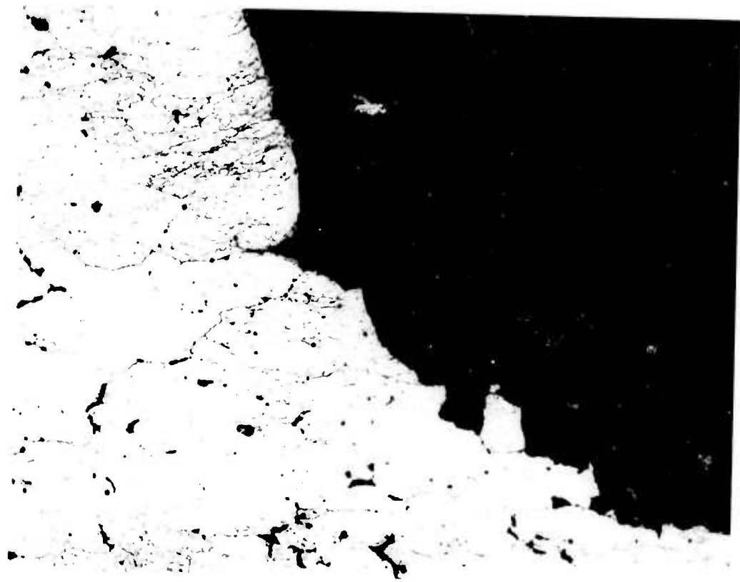
Figure 16. Fracture Profile of Tension Specimen 59 (Shown in Figure 12). Compared with Specimen 1A, a Larger Portion of the Fracture in Specimen 59 Was Transgranular. Keller's Etchant (200X).
