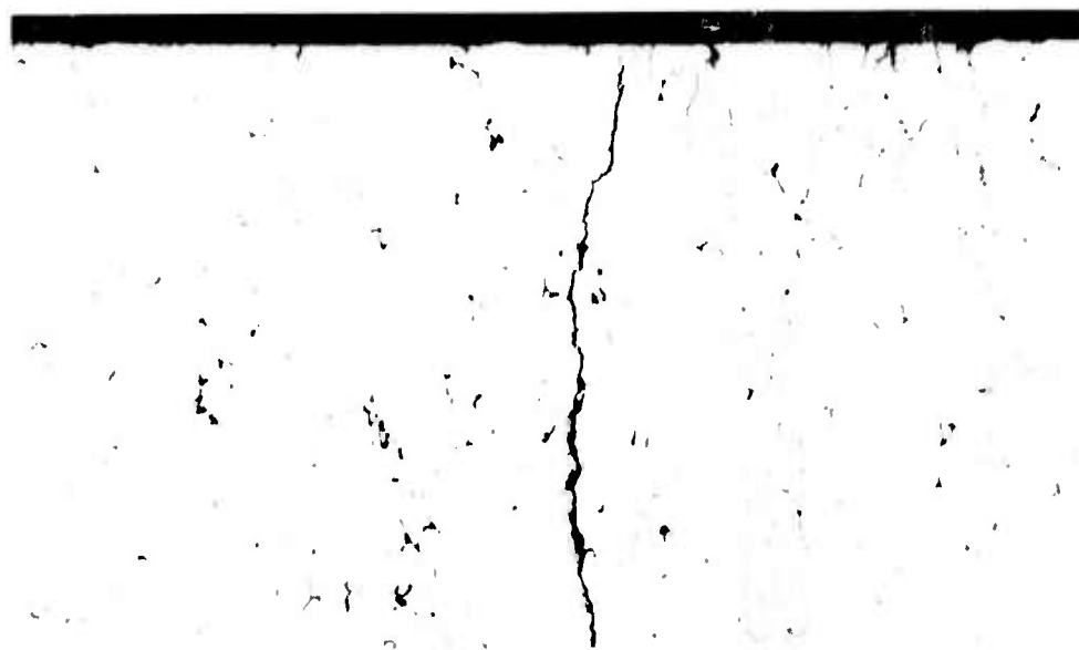
SPECIMEN 8B T6 + 10 HR AT 325°F 2.5 DAYS TO FAILURE
