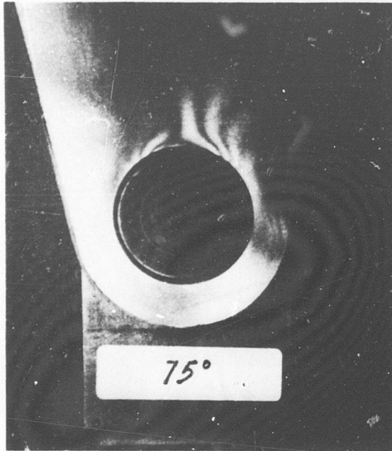
Figure 60g. Photoelastic Model of a Bolted Joint Loaded in Tension; 75^\circ Isoclines.
