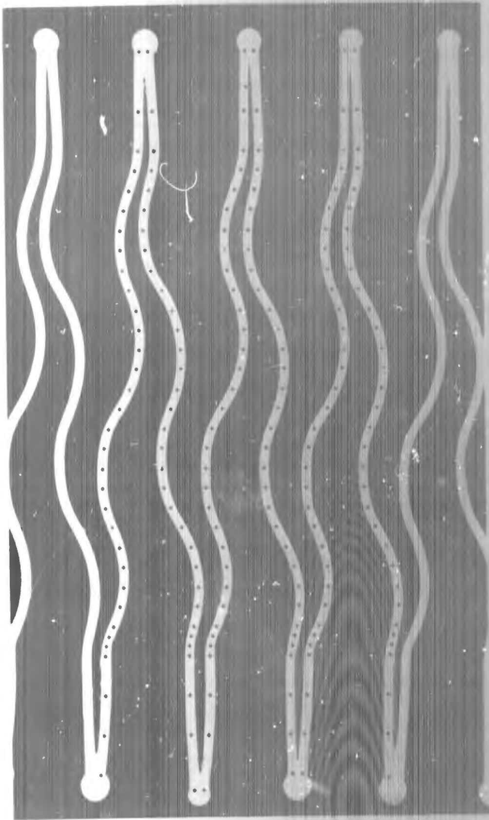
FIGURE 9-5. ENLARGED CROSS SECTIONAL VIEW OF A CONVENTIONAL 3.5-INCH WELDED BELLOWS JB-136
