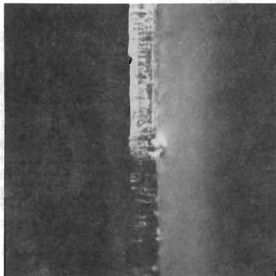
Figure V-23. Model 303 Seat With Embedded HB Particle (91X Plain Photo, Side Lighting)
