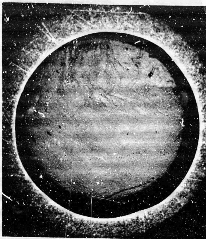
Figure 28. "Thornel" 50S-AI-11 Composite - Uncured. (25X)
