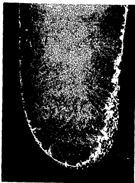
FIGURE 72. MICROSTRUCTURE OF G COATING ON RENE' 41 ALLOY AFTER HOT CORROSION TESTS AT 1650° F FOR 150 HOURS
