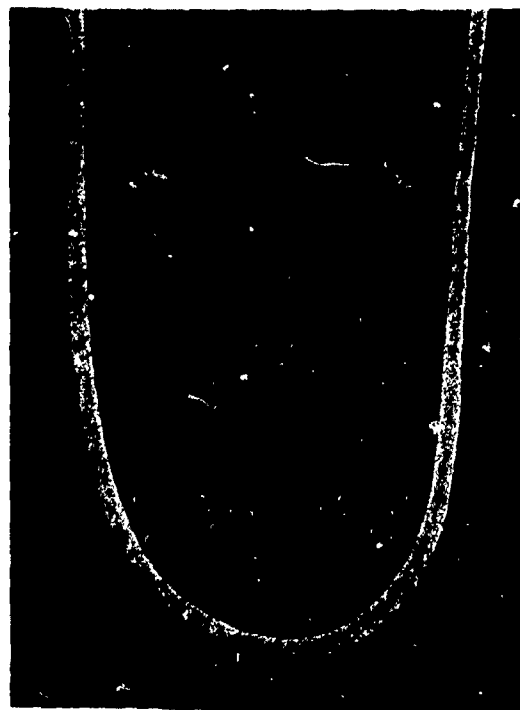
FIGURE 31. MICROSTRUCTURE OF AS-RECEIVED COATINGS; Coating A on B1900 Alloy
