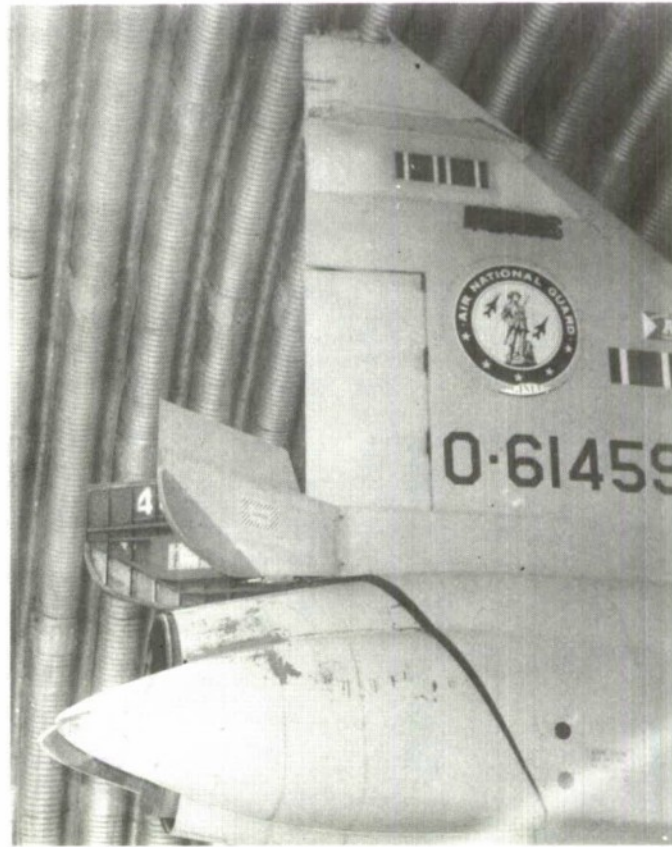
Figure 16. Tail Cone and Antenna Damage
