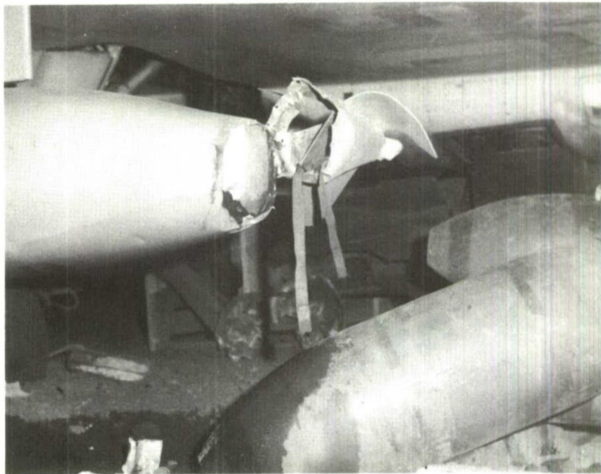
Figure 18. Damage to External Fuel Tank
