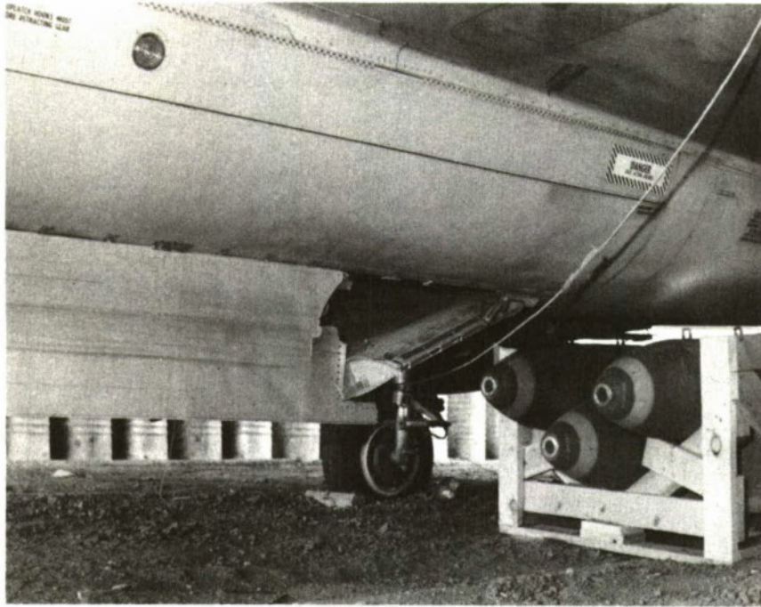
Figure 20. Armament Bay Door Damage
