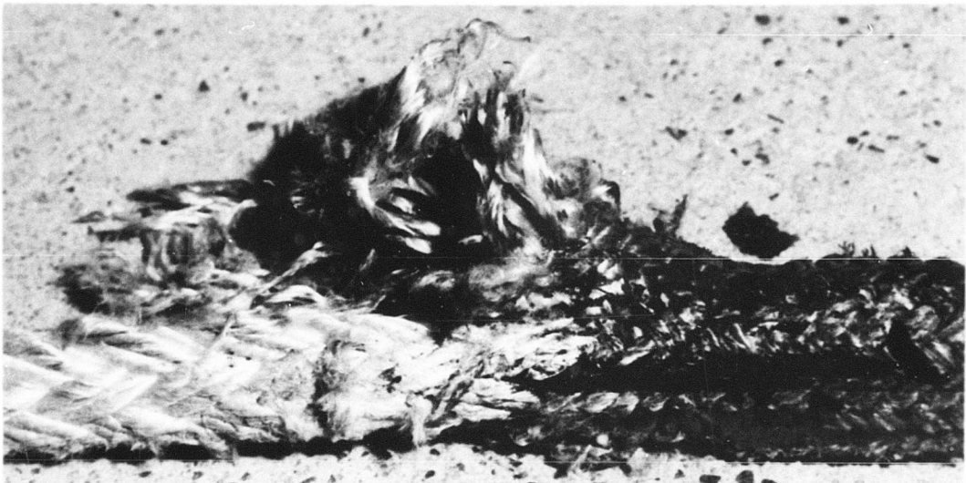
AAE PENDANT NO. 5 FOLLOWING 3 ARRESTMENTS AT 214, 219, AND 223 KNOTS (ALSO SEE FIGURE 7)
