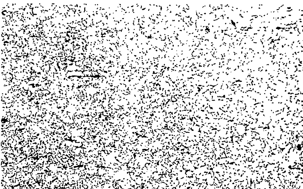
Figure 32 Neg. #2979-1967 Mag: 500X Mid-sidewall region of tempered case showing tempered martensite. Hardness R_c 26.
