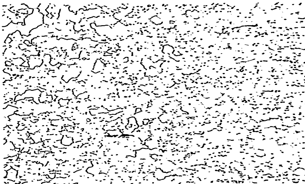
Figure 21 Neg. #2477-1967 Mag: 500X Upper sidewall of annealed second draw piece. The microstructure is equiaxed ferrite and spheroidal carbide. Hardness R_D 62-69.
