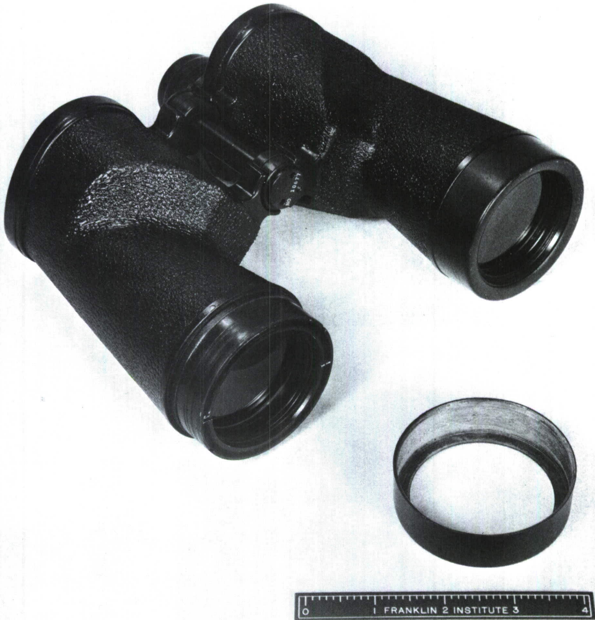
Figure 20 - M-17 Binoculars with Objective Ring Removed.
