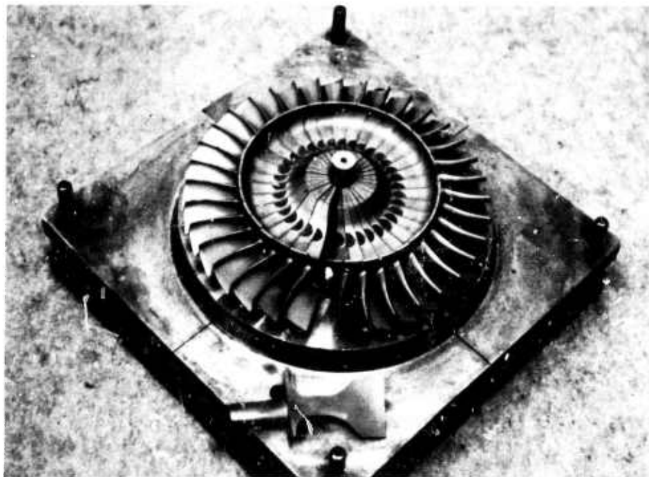
Figure 3.13 — Assembly of Molded Silicon Turbine Rotor Blades
