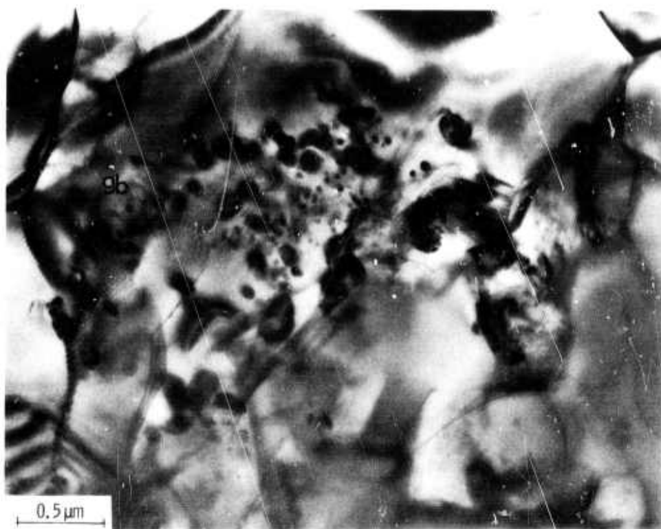
Figure 5.27 — Occasionally observed round impurities with associated strain fields. Also impurity particles in grain boundaries (g.b) 800 kV)
