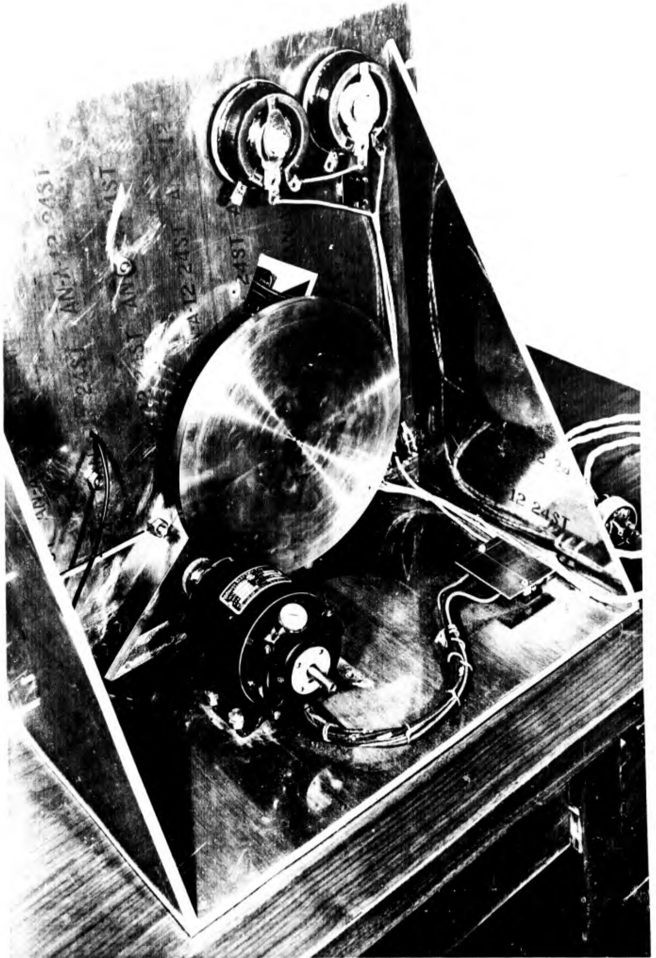
FIG. 10. REAR VIEW OF EXPERIMENTAL MAGNETIC RECORDING APPARATUS.
