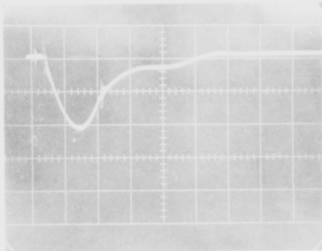
FIGURE 93 200,000 AMP CURRENT WAVESHAPES APPLIED TO CANOPY JOINT
