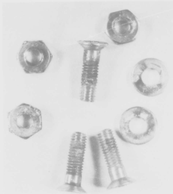
FIGURE 92 JOINT SCREWS DAMAGED BY 200,000 JOINT TEST
