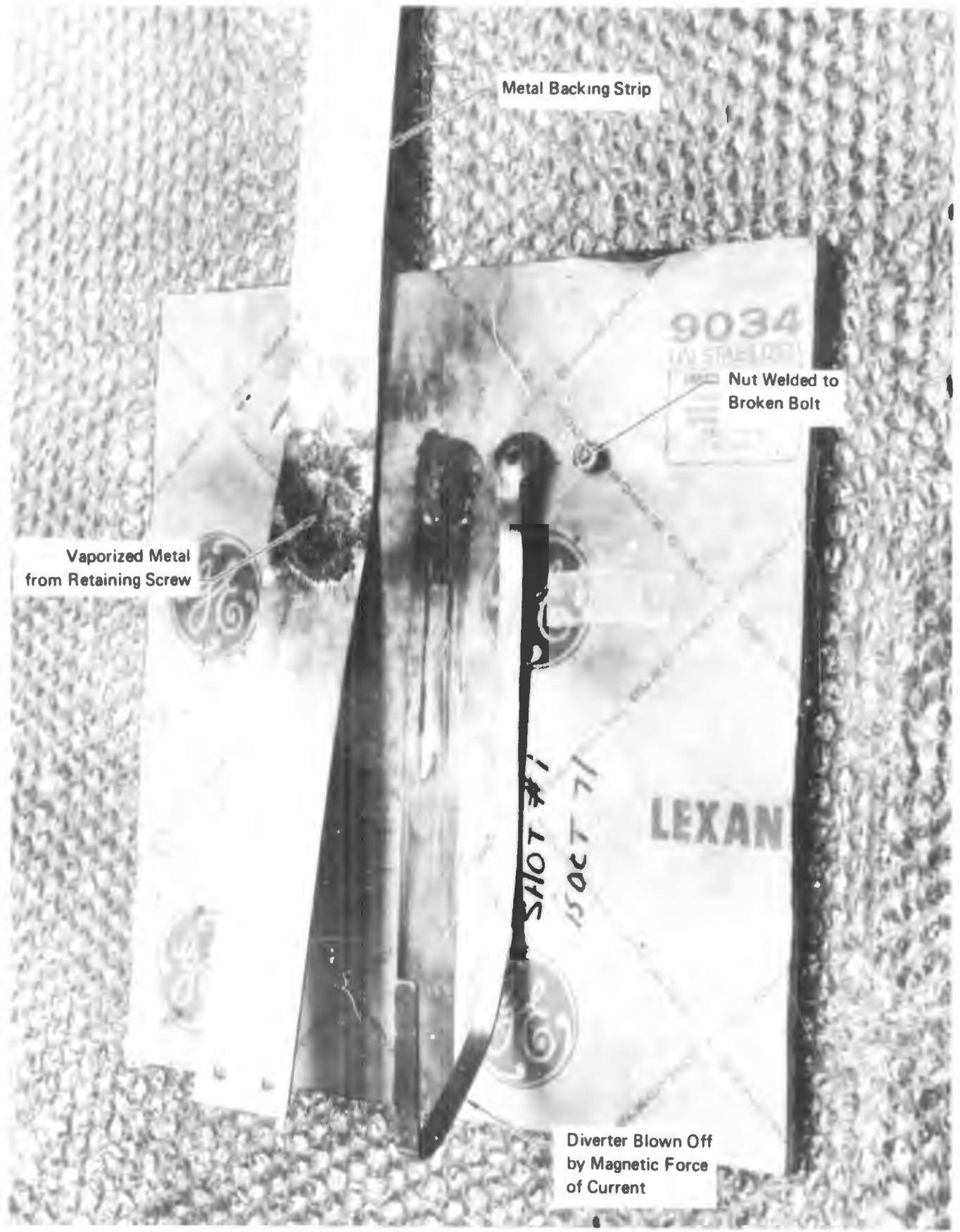
FIGURE 88 DIVERTER ATTACHMENT TYPE 1 AFTER 200,000 AMP TEST
