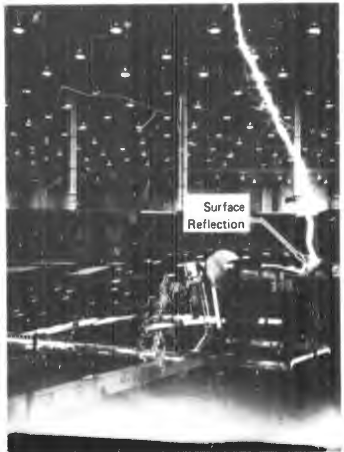
FIGURE 39 1.4 MV STRIKE TO UNPROTECTED CANOPY FROM 72 INCHES - SIDEVIEW
