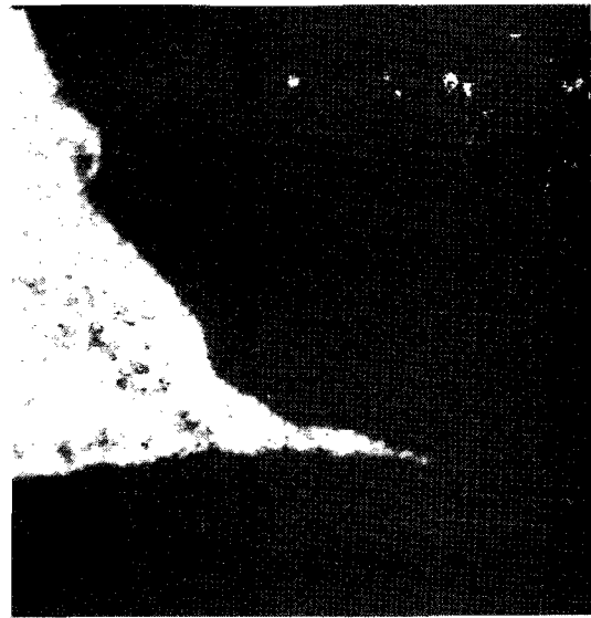
Figure I-25. Copper Microprobe Image Of Area Of Fig. I-24 (325X)
