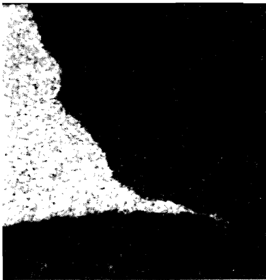
Figure I-26. Zinc Microprobe Image Of Area Of Fig. I-24 (325X)
