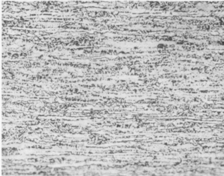
FIGURE 7.—EXAMPLE OF AS-RECEIVED EXTRUSION MICROSTRUCTURE, Ti-6Al-4V ANNEALED, SPECIMEN 2103-4-1 (MR = 0)
