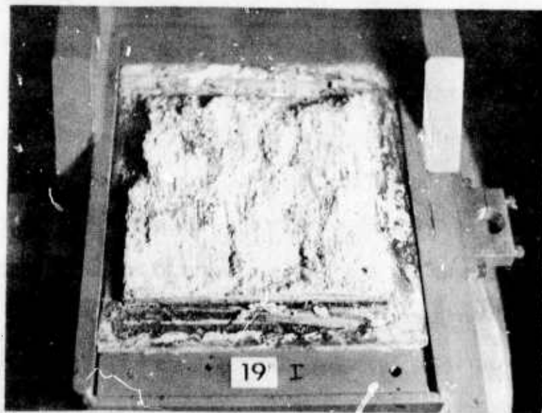
Figure 36. Specimen 19p - natural joint surface and after shearing at \sigma_n = 1521 . Specimen size 6x6 inch.
