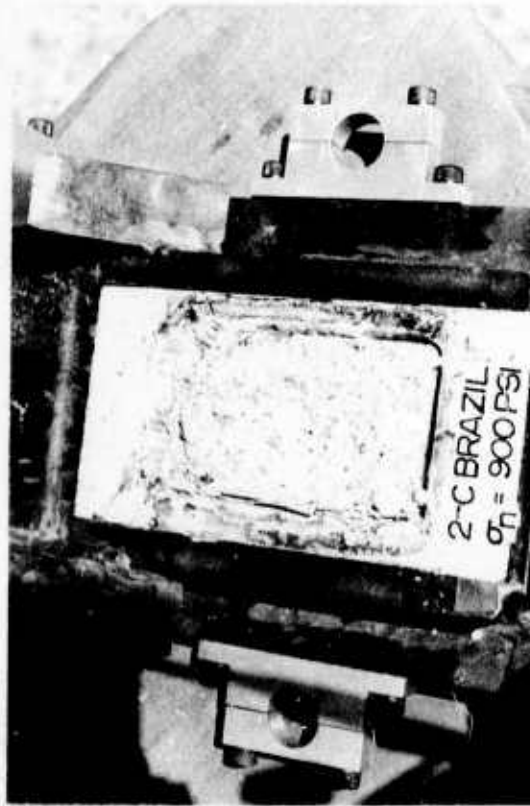
Figure 44. Brazil Tests - Surface modification as a function of normal stress. Specimen size 2.125x2.80 in. Note development of slickensides and gouge with normal stress.
