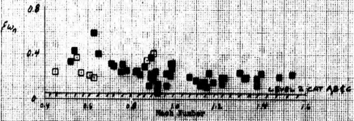
Figure 59. Flight Test Data: Roll Characteristics (Transonic and Supersonic - SAS OFF)
