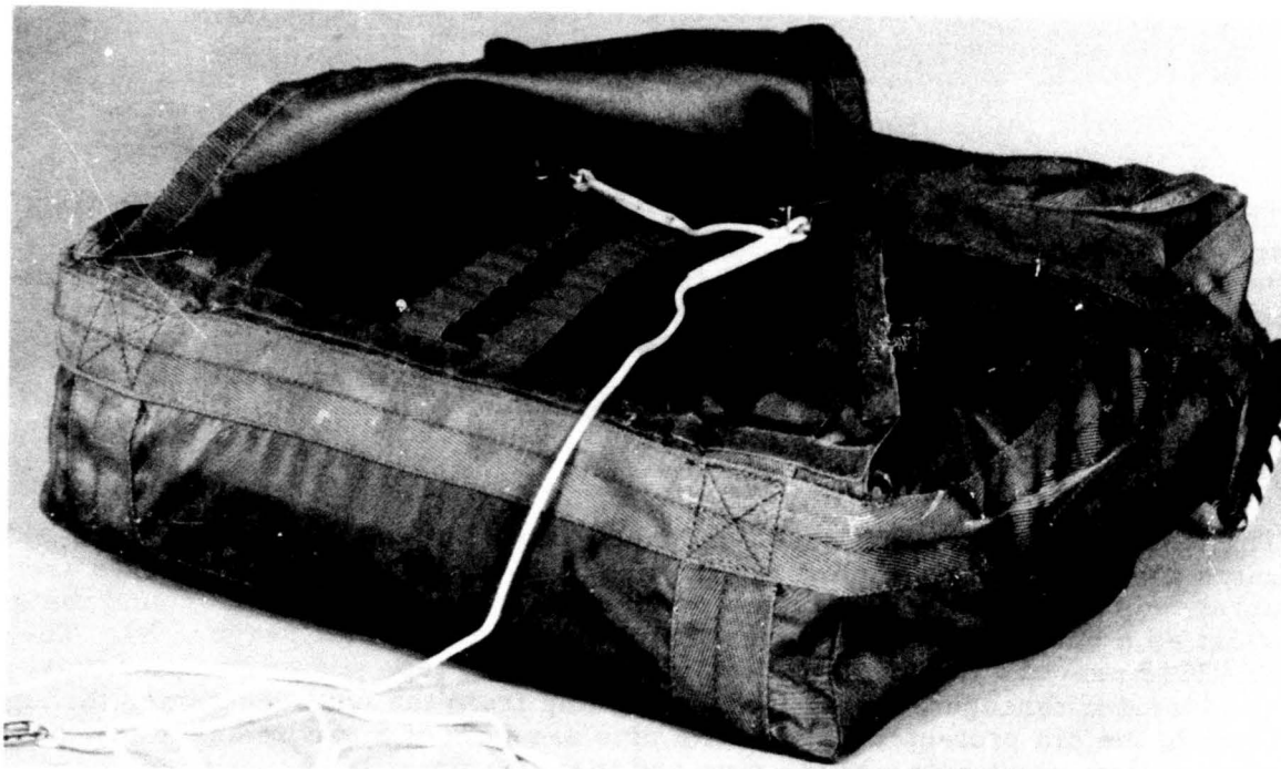
FIGURE 85. RIPCORDER PINS THROUGH RING ASSEMBLY AND CORD LOOPS
