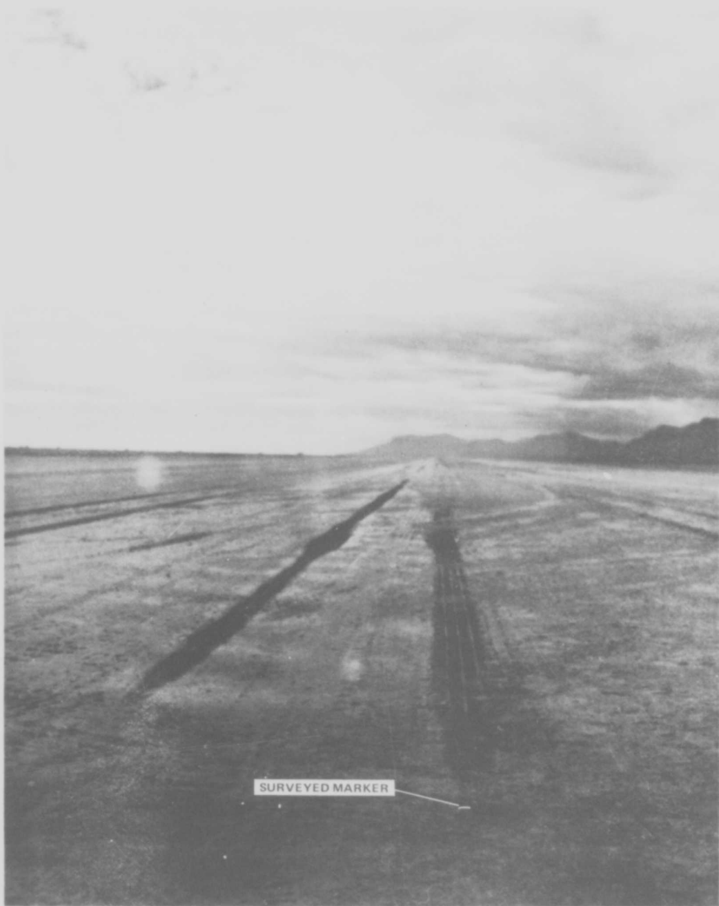
Figure 10-5 621 B Aircraft "Footprint" at Touchdown
