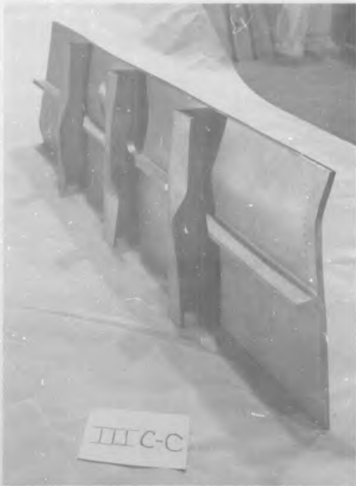
FIGURE 18. -POSTFAILURE PHOTOGRAPH OF III C-C CRIPPLING PANEL
