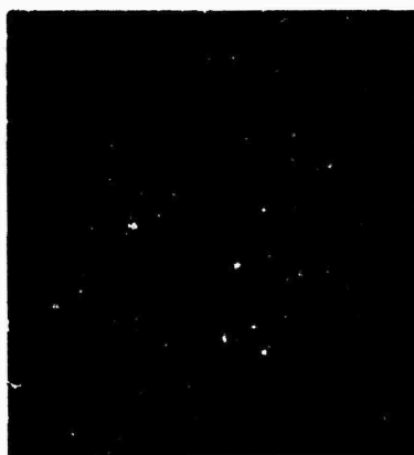
Fig. 28. RCA C70021AEP2 tube with 1-h exposure. The Baum image is the result of phosphor persistence in the first dynode. The ion dark emission is seen to strongly affect the noise of the photographic image. The presence of electron dark emission is barely discernible in the reproduction.
