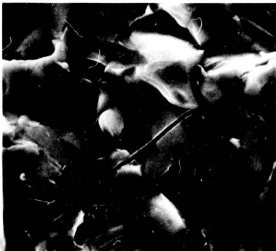
Figure 5.48 Transgranular Crack on the Fracture Surface of Reaction Sintered Silicon Carbide
