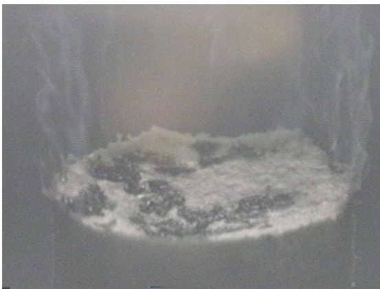
b. HMX2 burning at 1.5 MPa. hmx2\hmx215m.avi hmx2\hmx215m.mov
