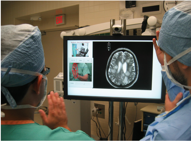
Fig. 4.3: Gestix operated by a surgeon in the operating room at the Washington Hospital Center.
