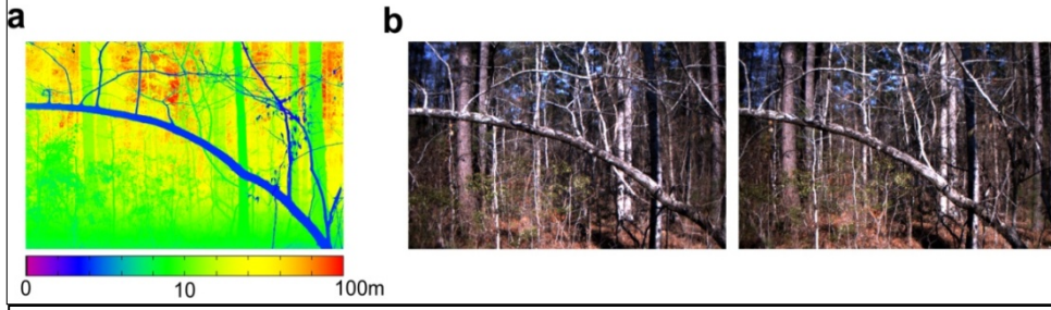
Fig. 1. Image registration. (a), Range image of a natural scene; the distance is indicated by color-coding. (b), A pair of stereoscopic images of the same scene.
