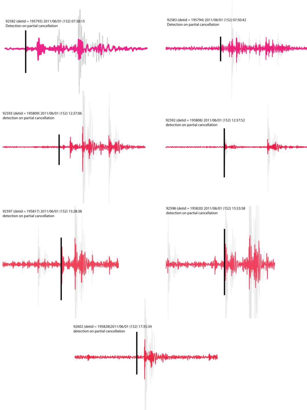
Figure 19. Instances in which the framework produced detections on incompletely cancelled icequake signals. The magenta traces are the post-cancellation signals, and the light gray shows the original signal. The detection time is indicated by the vertical black line.
