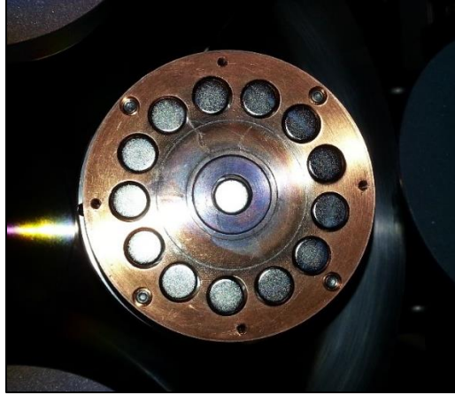
Figure 6.2 - Sputter gun's magnet array after TiO deposition
