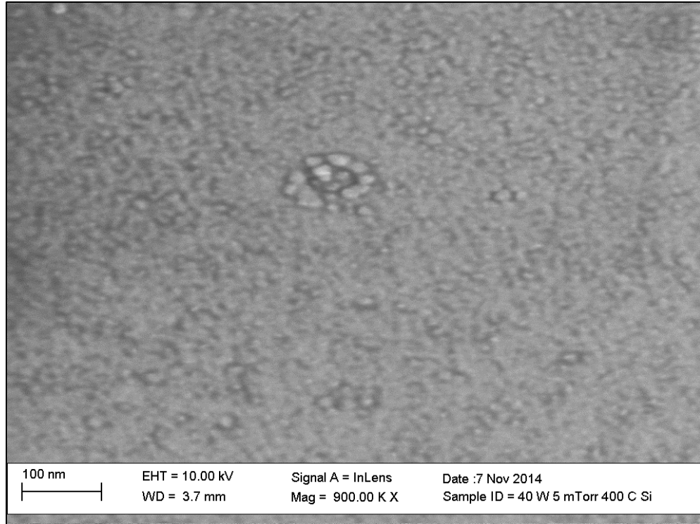
Figure 5.16 - Temperature deposition at 400°C on Silicon, grains (12nm and 15nm)
