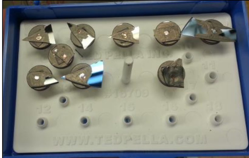
Figure 3.8 - Samples prepared with copper grid and graphite paste
