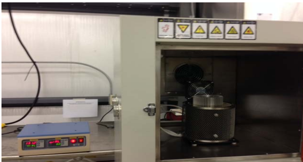
Figure 4: High temperature/pressure hydrothermal reactor
