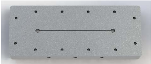
Figure 1 Sketch of the 1 mm \times 1 mm groove machined in the aluminum plate.
