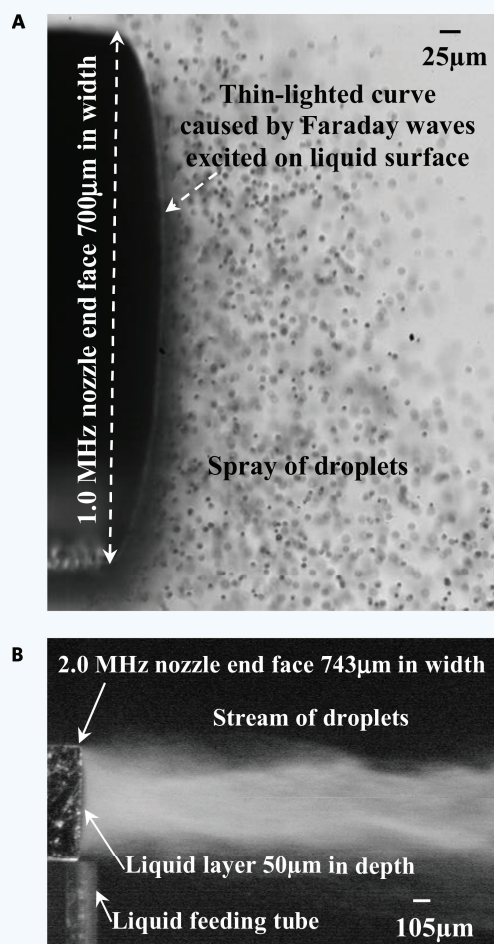
Figure 4 Stream of droplets ejected from the liquid layer resting on the end face of the nozzle tip: (A) High-speed photograph ( 10^4 frame/sec, Vision Research Model Phantom ® v7.2) with short depth of focus for droplets stream at output rate of 40 \mu\text{L}/\text{min} with 1.0 MHz nozzle. (B) CCD image (20 frame/sec) of droplets stream at output rate of 350 \mu\text{L}/\text{min} and electrical drive power of 0.27 W with optimized 2.0 MHz nozzle. Note that the scale bars in (A) and (B) are 25 \mu\text{m} and 105 \mu\text{m} , respectively.
