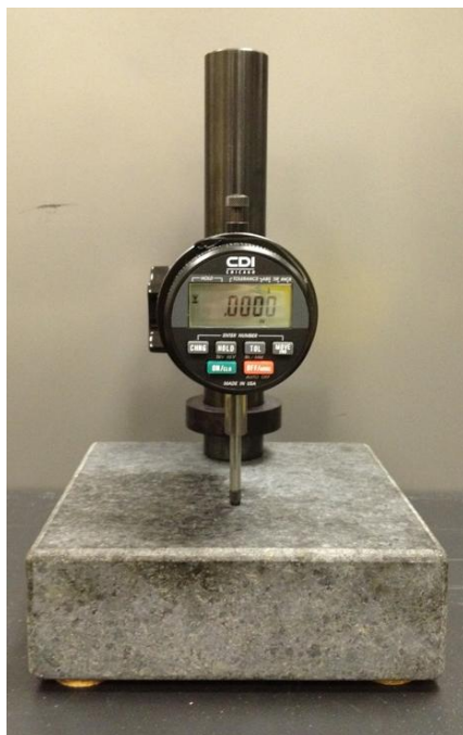
Figure 5. Micrometer Used for Measuring Cross Sectional Thickness
