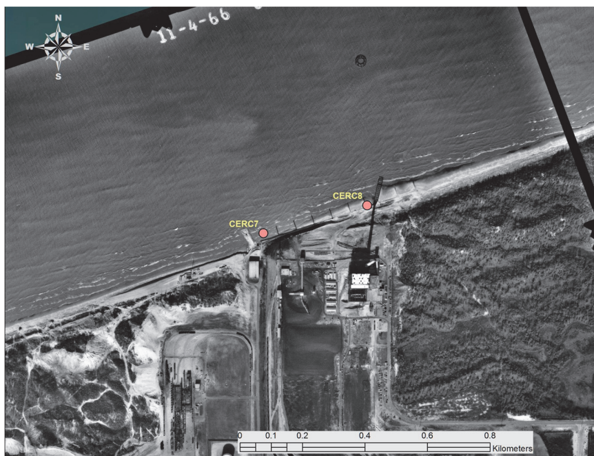
Fig. 5. Shoreline at initial stage of Burns Waterway Harbor construction, 4 November 1966. Note bulkhead near CERC7. The circle in the lake is the BGS cooling water intake.
