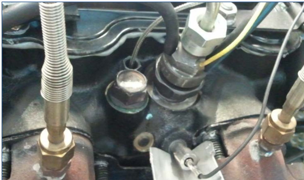
Figure 5. GEP 6.5LT Cylinder Pressure Transducers and Instrumented Injector
