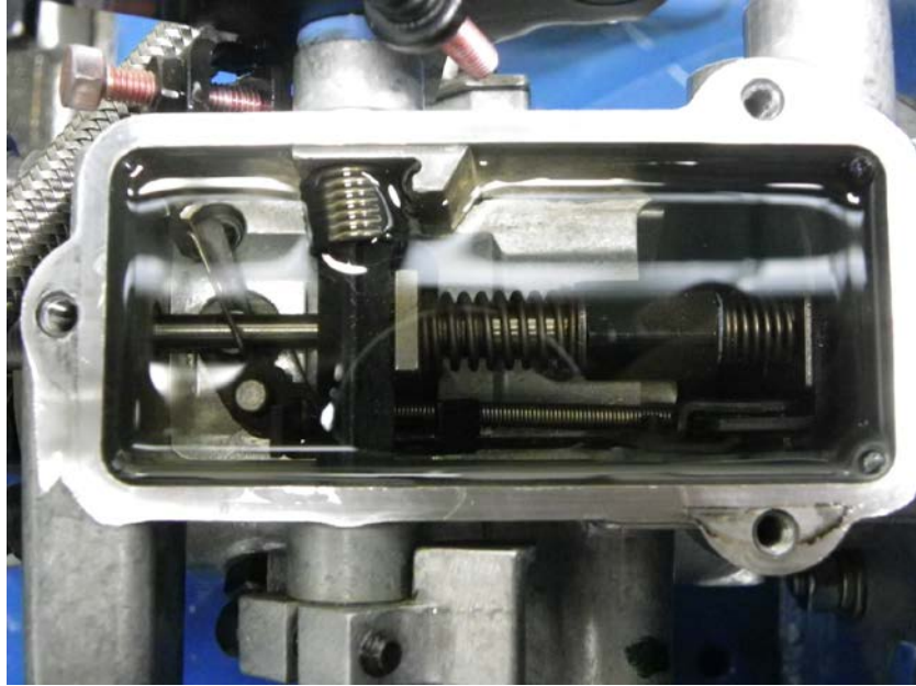
Figure 12. Pump SN:16756536 Governor Assembly with 1000-Hours Testing with ATJ/JP-8 Fuel
