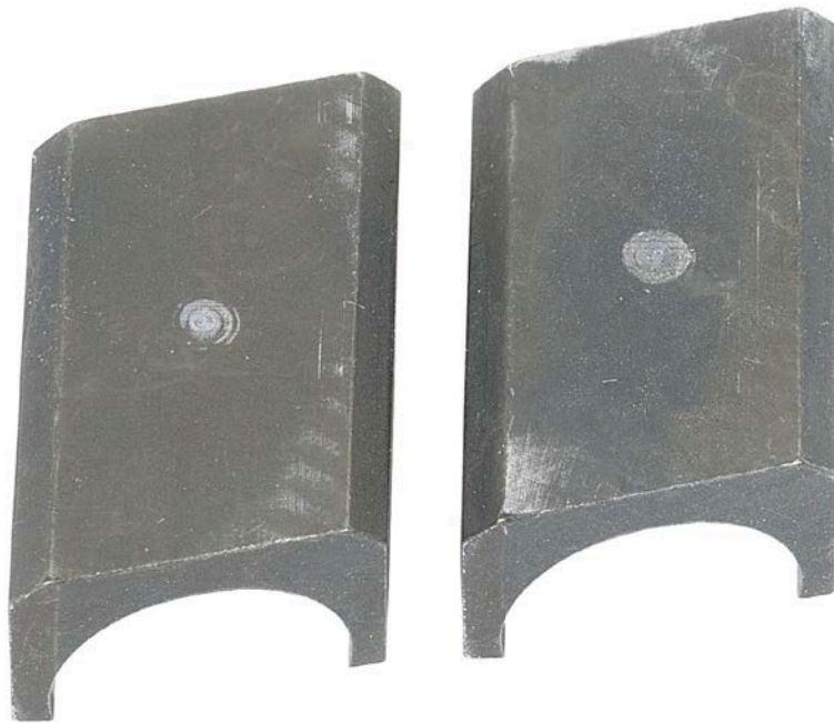
Figure 73. Pump SN:16756538 Roller Shoe before Testing with 25/75 ATJ/JP-8 Fuel with 24-ppm CI/LI
