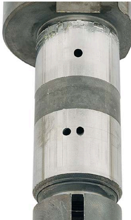
Figure 15. Pump SN:16756534 Distributor Rotor with 251-hours Testing with 25/75 ATJ/JP-8 Fuel with 9-ppm CI/LI
