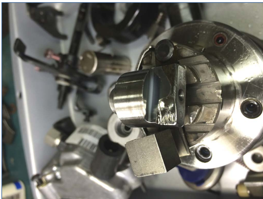
Figure 4. Pump SN:16756534 Showing Fractured Drive Shaft, Drive Tang Wear, and Rotor Distress at 251-hours with 25/75 ATJ/JP-8 Fuel with 9-ppm CI/LI at 77 °C Inlet Temperature
