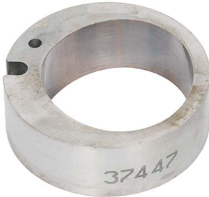
Figure 26. Pump SN:16756534 Transfer Pump Liner with 251-hours Testing with 25/75 ATJ/JP-8 Fuel with 9-ppm CI/LI
