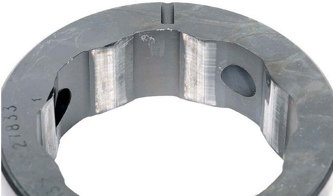
Figure 58. Pump SN:16756536 Cam Ring with 1000-Hours Testing with 25/75 ATJ/JP-8 Fuel with 24-ppm CI/LI
