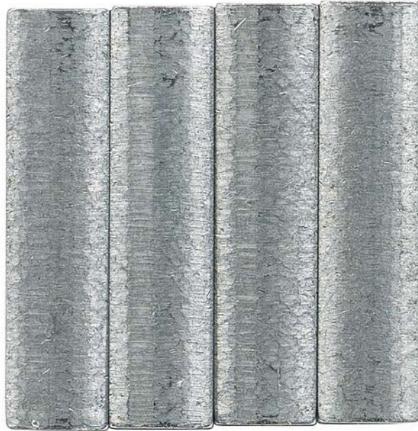
Figure 63. Pump SN:16756536 Transfer Pump Blade Edges before Testing with 25/75 ATJ/JP-8 Fuel with 24-ppm CI/LI
