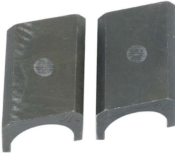
Figure 55. Pump SN:16756536 Roller Shoe before Testing with 25/75 ATJ/JP-8 Fuel with 24-ppm CI/LI
