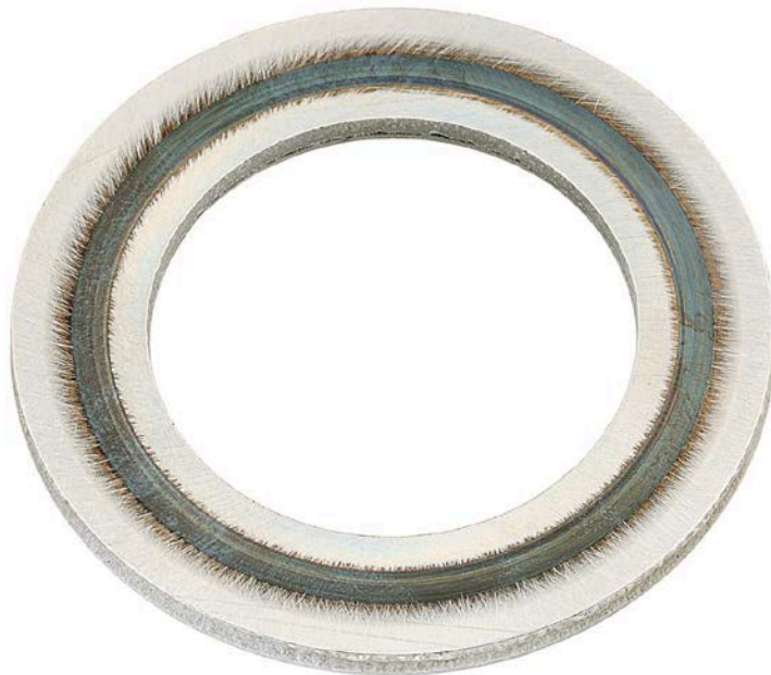
Figure 78. Pump SN:16756538 Thrust Washer with 1000-Hours Testing with 25/75 ATJ/JP-8 Fuel with 24-ppm CI/LI
