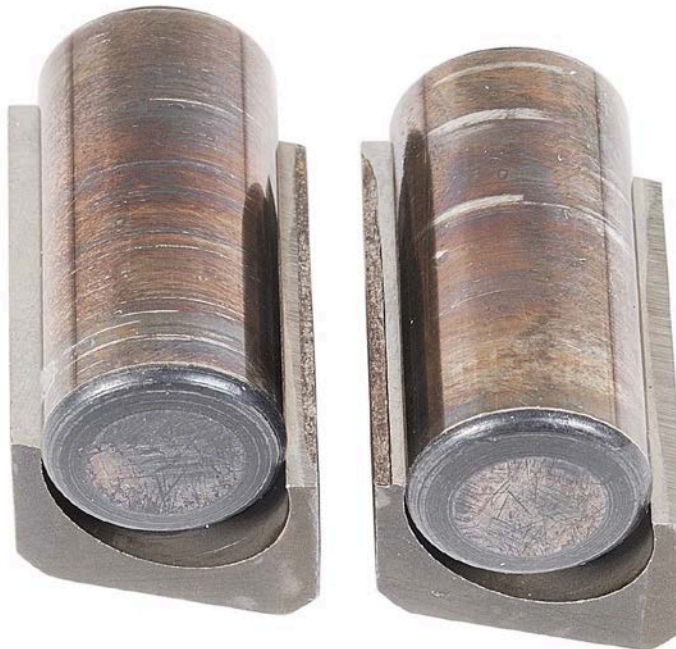
Figure 36. Pump SN:16756535 Rollers and Shoe with 389-hours Testing with 25/75 ATJ/JP-8 Fuel with 9-ppm CI/LI
