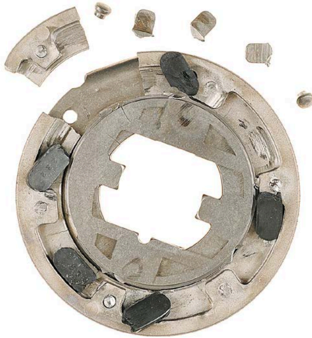
Figure 16. Pump SN:16756534 Governor Weight Cage Breakage with 251-hours Testing with 25/75 ATJ/JP-8 Fuel with 9-ppm CI/LI
