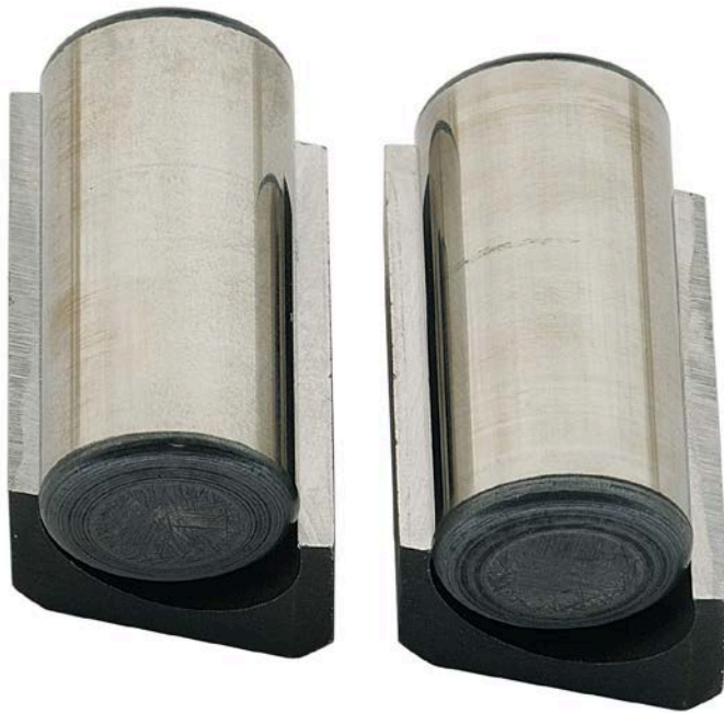
Figure 71. Pump SN:16756538 Rollers and Shoe before Testing with 25/75 ATJ/JP-8 Fuel with 24-ppm CI/LI
