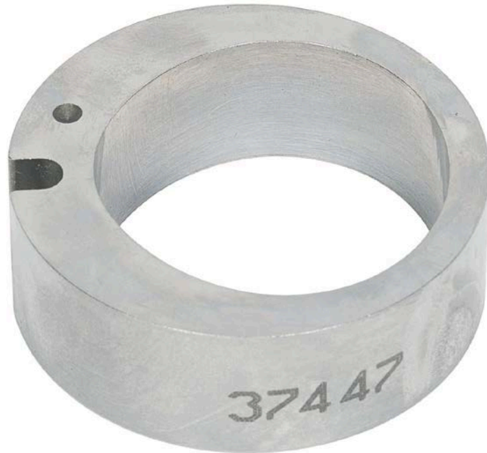
Figure 79. Pump SN:16756538 Transfer Pump Liner before Testing with 25/75 ATJ/JP-8 Fuel with 24-ppm CI/LI
