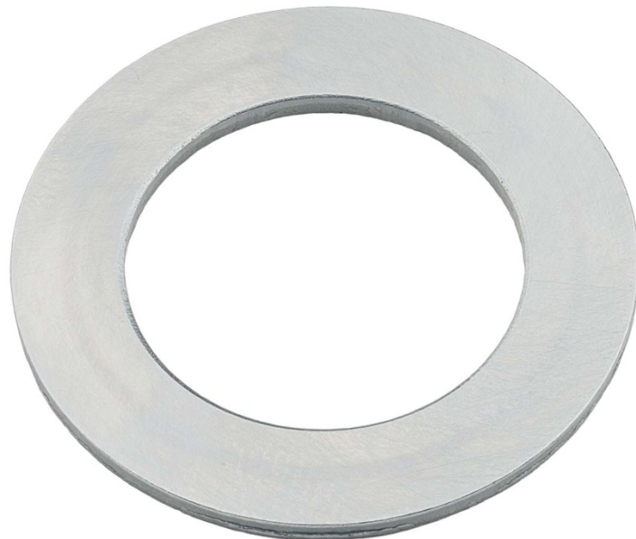
Figure 23. Pump SN:16756534 Thrust Washer before Testing with 25/75 ATJ/JP-8 Fuel with 9-ppm CI/LI
