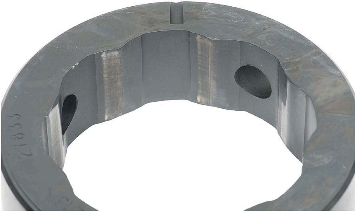
Figure 57. Pump SN:16756536 Cam Ring before Testing with 25/75 ATJ/JP-8 Fuel with 24-ppm CI/LI
