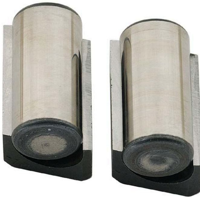
Figure 53. Pump SN:16756536 Rollers and Shoe before Testing with 25/75 ATJ/JP-8 Fuel with 24-ppm CI/LI
