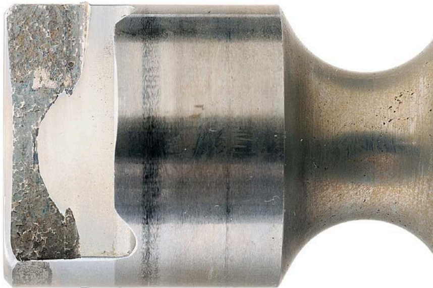
Figure 86. Pump SN:16756538 Driveshaft Drive Tang with 1000-Hours Testing with 25/75 ATJ/JP-8 Fuel with 24-ppm CI/LI
