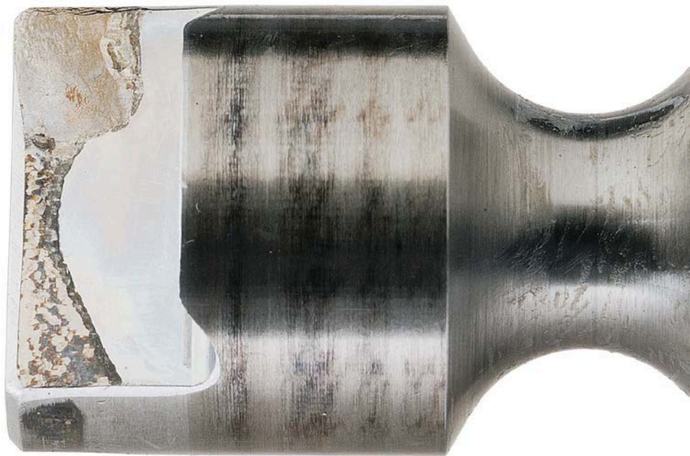
Figure 50. Pump SN:16756535 Driveshaft Drive Tang with 389-Hours Testing with 25/75 ATJ/JP-8 Fuel with 9-ppm CI/LI
