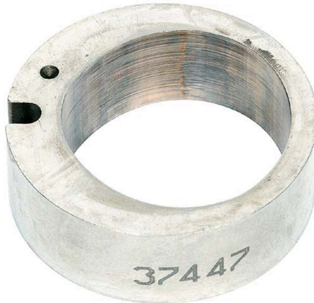
Figure 80. Pump SN:16756538 Transfer Pump Liner with 1000-Hours Testing with 25/75 ATJ/JP-8 Fuel with 24-ppm CI/LI
