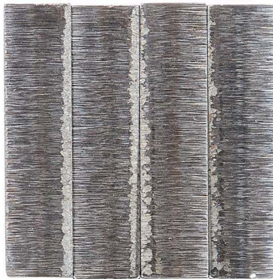
Figure 64. Pump SN:16756536 Transfer Pump Blade Edges with 1000-Hours Testing with 25/75 ATJ/JP-8 Fuel with 24-ppm CI/LI
