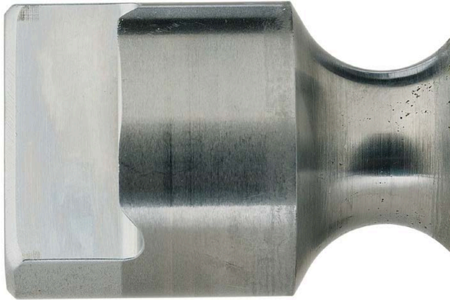
Figure 85. Pump SN:16756538 Driveshaft Drive Tang before Testing with 25/75 ATJ/JP-8 Fuel with 24-ppm CI/LI
