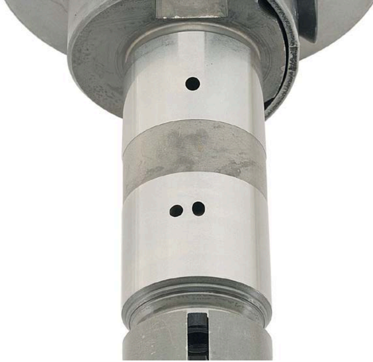
Figure 51. Pump SN:16756536 Distributor Rotor before Testing with 25/75 ATJ/JP-8 Fuel with 24-ppm CI/LI
