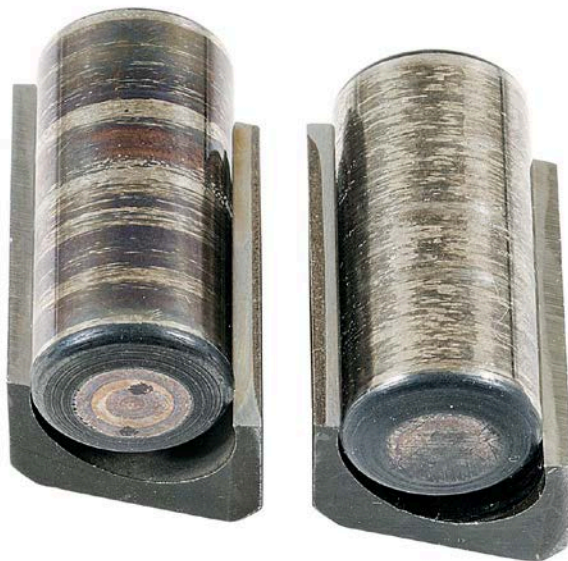
Figure 72 Pump SN:16756538 Rollers and Shoe with 1000-Hours Testing with 25/75 ATJ/JP-8 Fuel with 24-ppm CI/LI
