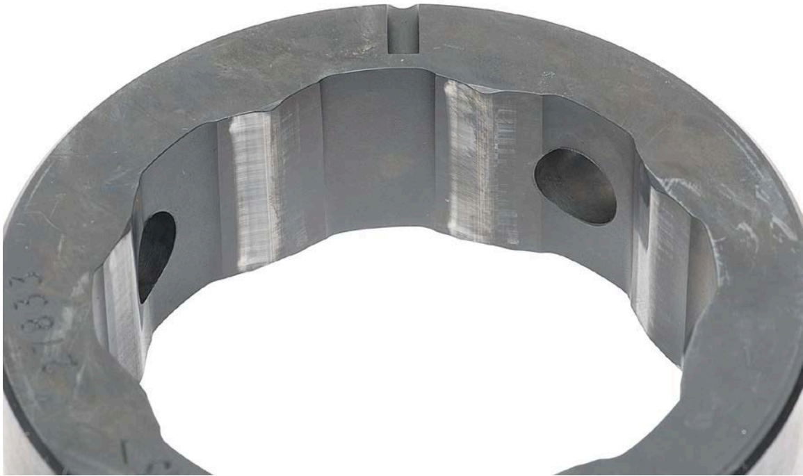
Figure 75. Pump SN:16756538 Cam Ring before Testing with 25/75 ATJ/JP-8 Fuel with 24-ppm CI/LI
