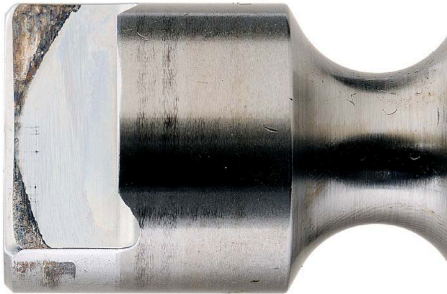
Figure 68. Pump SN:16756536 Driveshaft Drive Tang with 1000-Hours Testing with 25/75 ATJ/JP-8 Fuel with 24-ppm CI/LI
