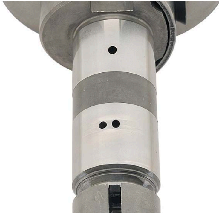
Figure 14. Pump SN:16756534 Distributor Rotor before Testing with 25/75 ATJ/JP-8 Fuel with 9-ppm CI/LI
