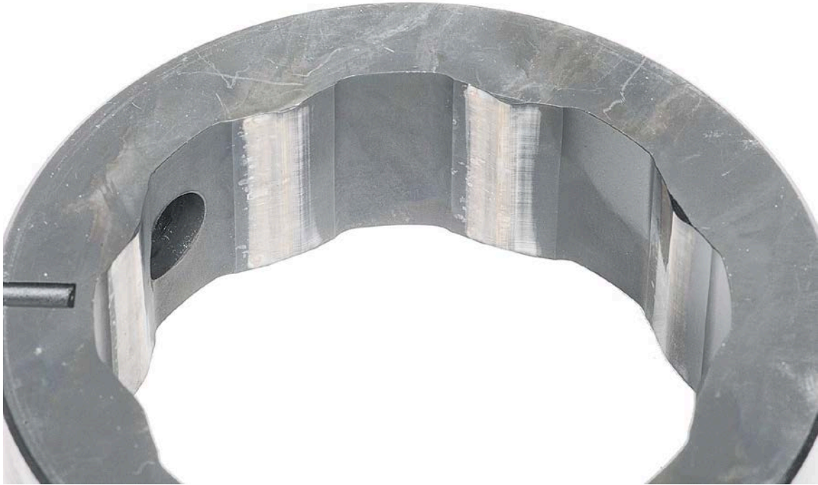
Figure 22. Pump SN:16756534 Cam Ring with 251-hours Testing with 25/75 ATJ/JP-8 Fuel with 9-ppm CI/LI
