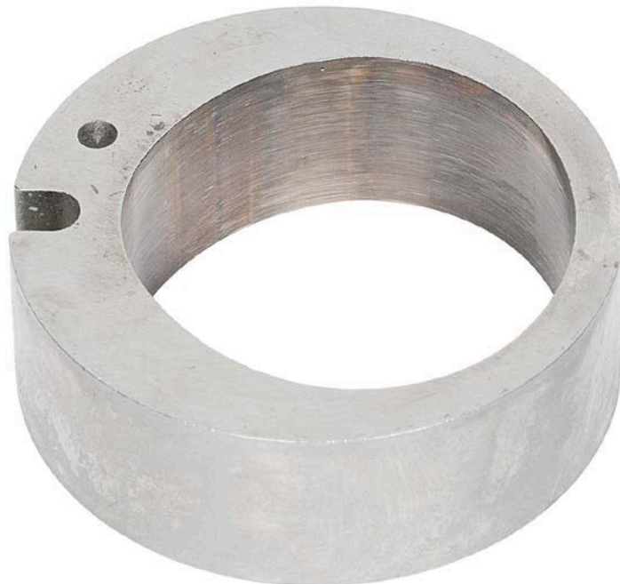
Figure 44. Pump SN:16756535 Transfer Pump Liner with 389-hours Testing with 25/75 ATJ/JP-8 Fuel with 9-ppm CI/LI
