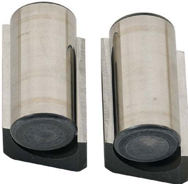
Figure 17. Pump SN:16756534 Rollers and Shoe before Testing with 25/75 ATJ/JP-8 Fuel with 9-ppm CI/LI
