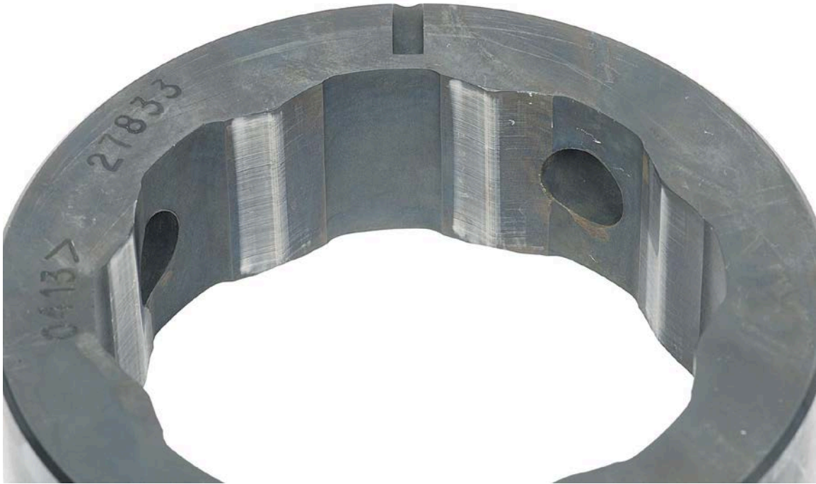
Figure 39. Pump SN:16756535 Cam Ring Before Testing with 25/75 ATJ/JP-8 Fuel with 9-ppm CI/LI
