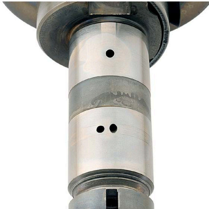
Figure 70. Pump SN:16756538 Distributor Rotor with 1000-Hours Testing with 25/75 ATJ/JP-8 Fuel with 24-ppm CI/LI
