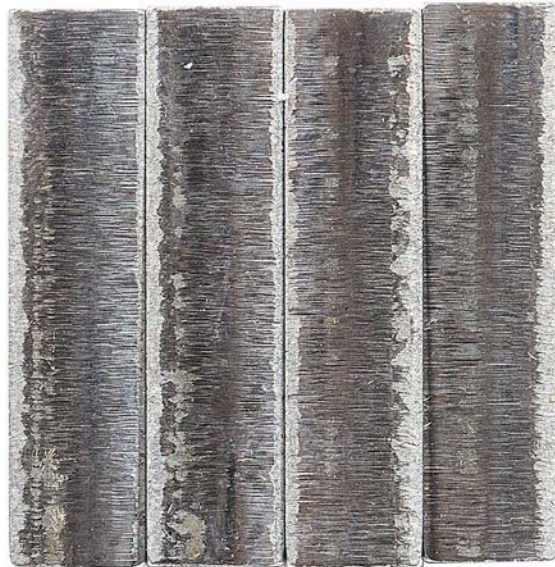
Figure 82. Pump SN:16756538 Transfer Pump Blade Edges with 1000-Hours Testing with 25/75 ATJ/JP-8 Fuel with 24-ppm CI/LI
