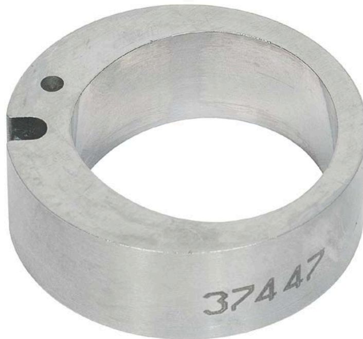
Figure 25. Pump SN:16756534 Transfer Pump Liner before Testing with 25/75 ATJ/JP-8 Fuel with 9-ppm CI/LI
