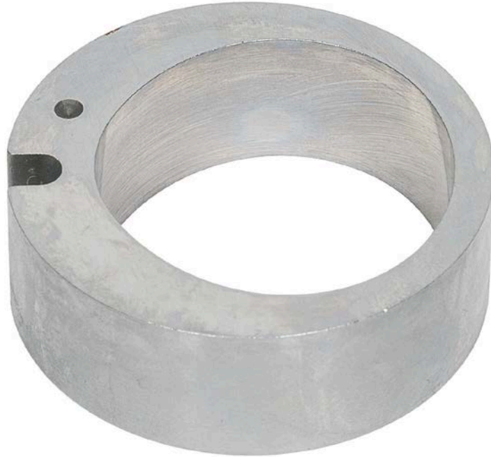
Figure 61. Pump SN:16756536 Transfer Pump Liner before Testing with 25/75 ATJ/JP-8 Fuel with 24-ppm CI/LI
