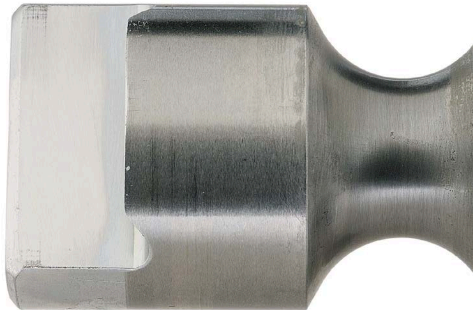
Figure 31. Pump SN:16756534 Driveshaft Drive Tang before Testing with 25/75 ATJ/JP-8 Fuel with 9-ppm CI/LI
