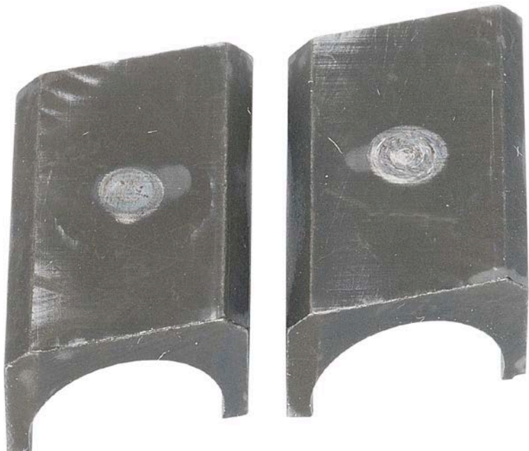
Figure 38. Pump SN:16756535 Roller Shoe with 389-hours Testing with 25/75 ATJ/JP-8 Fuel with 9-ppm CI/LI
