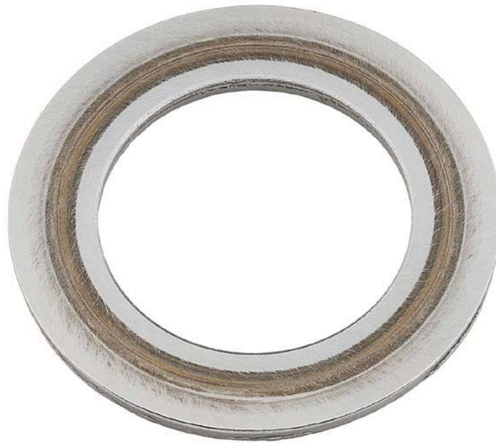
Figure 24. Pump SN:16756534 Thrust Washer with 251-hours Testing with 25/75 ATJ/JP-8 Fuel with 9-ppm CI/LI
