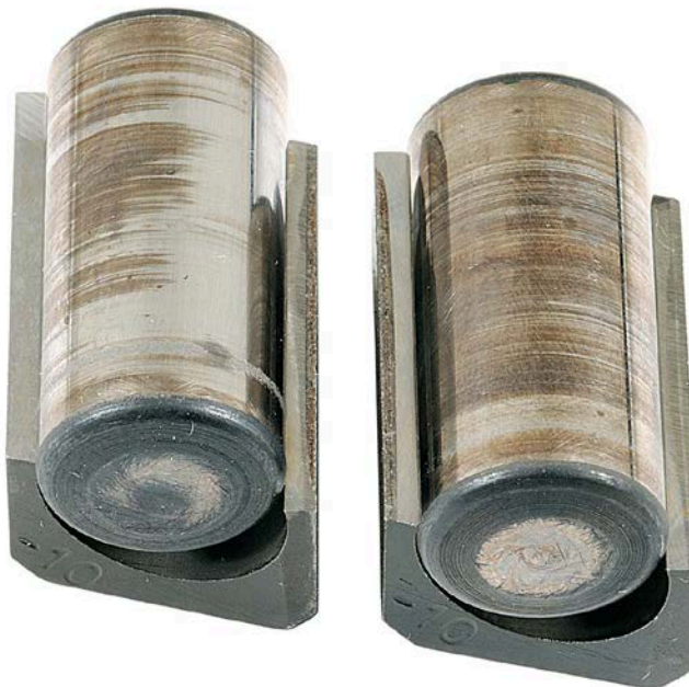
Figure 54. Pump SN:16756536 Rollers and Shoe with 1000-Hours Testing with 25/75 ATJ/JP-8 Fuel with 24-ppm CI/LI
