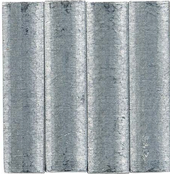
Figure 81. Pump SN:16756538 Transfer Pump Blade Edges before Testing with 25/75 ATJ/JP-8 Fuel with 24-ppm CI/LI
