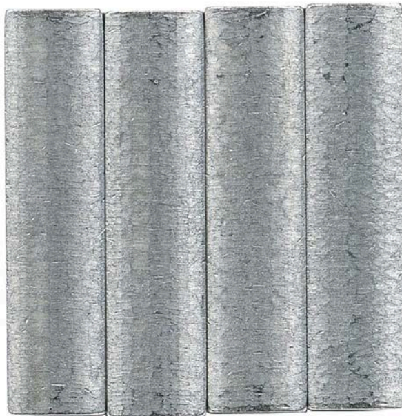
Figure 27. Pump SN:16756534 Transfer Pump Blade Edges before Testing with 25/75 ATJ/JP-8 Fuel with 9-ppm CI/LI
