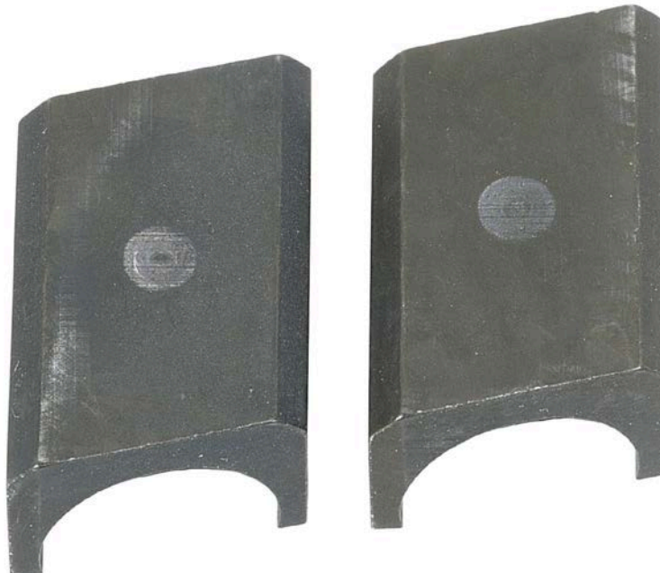
Figure 19. Pump SN:16756534 Roller Shoe before Testing with 25/75 ATJ/JP-8 Fuel with 9-ppm CI/LI
