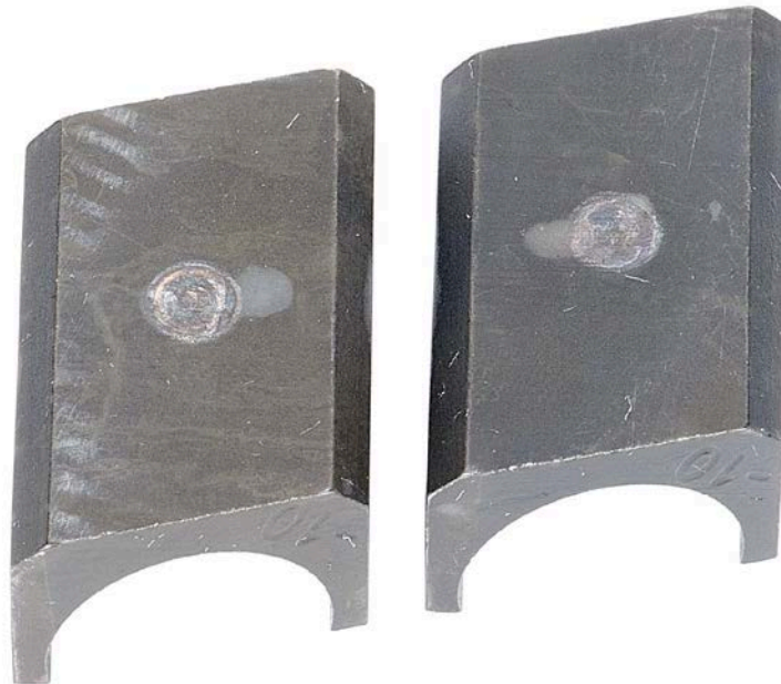
Figure 56. Pump SN:16756536 Roller Shoe with 1000-Hours Testing with 25/75 ATJ/JP-8 Fuel with 24-ppm CI/LI
