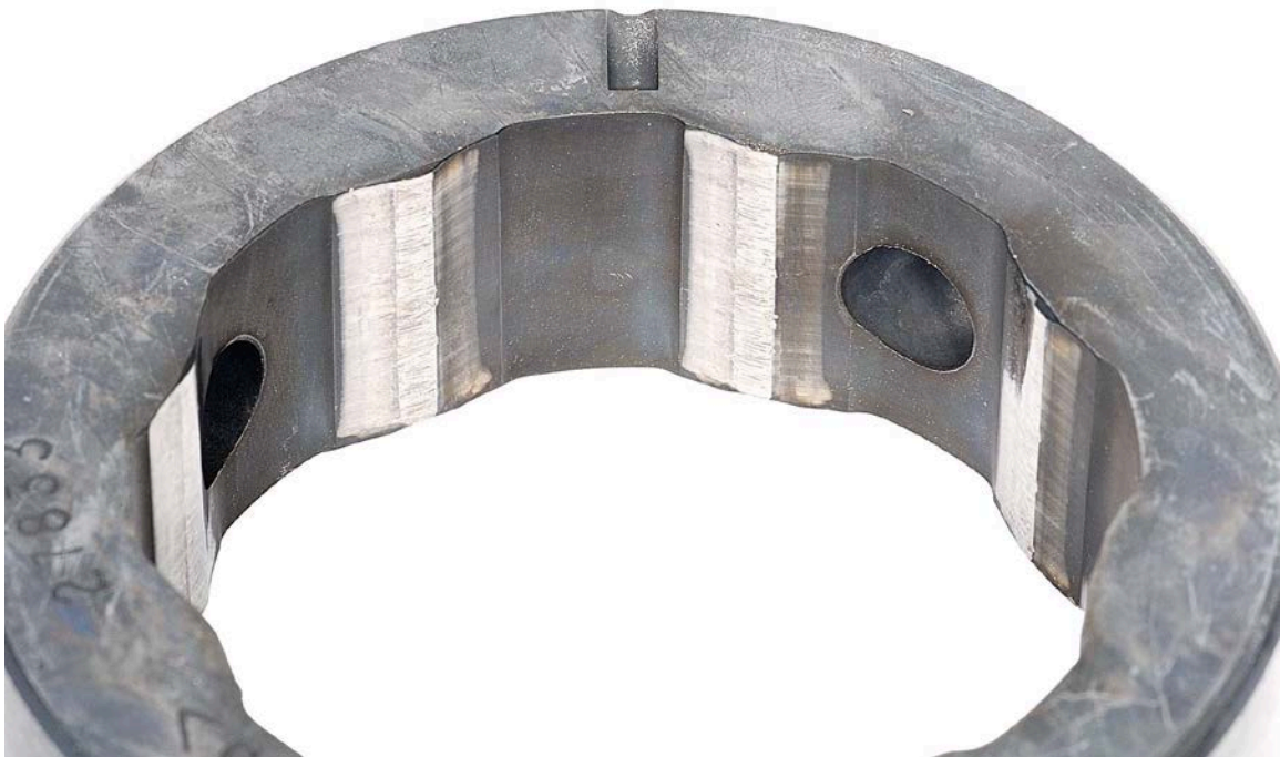
Figure 76. Pump SN:16756538 Cam Ring with 1000-Hours Testing with 25/75 ATJ/JP-8 Fuel with 24-ppm CI/LI
