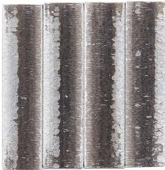
Figure 28. Pump SN:16756534 Transfer Pump Blade Edges with 251-hours Testing with 25/75 ATJ/JP-8 Fuel with 9-ppm CI/LI
