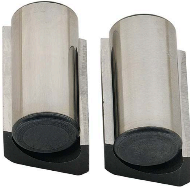
Figure 35. Pump SN:16756535 Rollers and Shoe Condition before Testing with 25/75 ATJ/JP-8 Fuel with 9-ppm CI/LI
