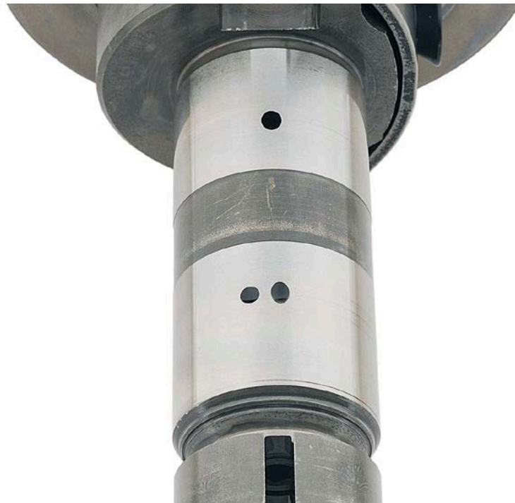
Figure 34. Pump SN:16756535 Distributor Rotor with 389-hours Testing with 25/75 ATJ/JP-8 Fuel with 9-ppm CI/LI
