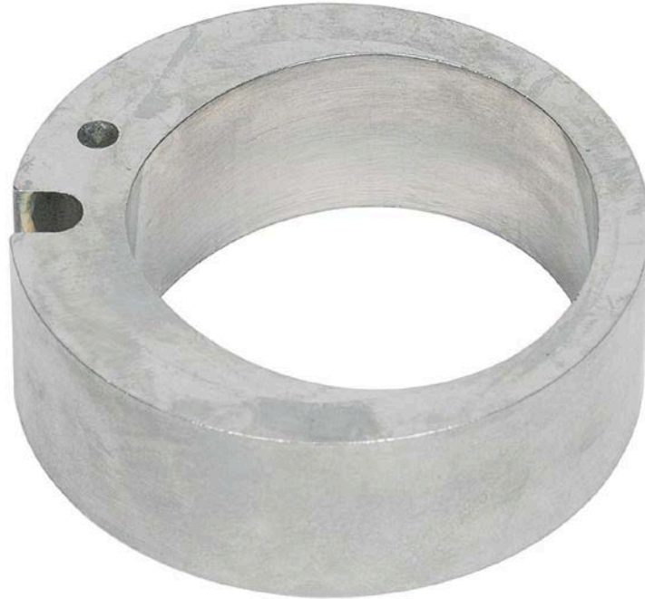
Figure 43. Pump SN:16756535 Transfer Pump Liner before Testing with 25/75 ATJ/JP-8 Fuel with 9-ppm CI/LI
