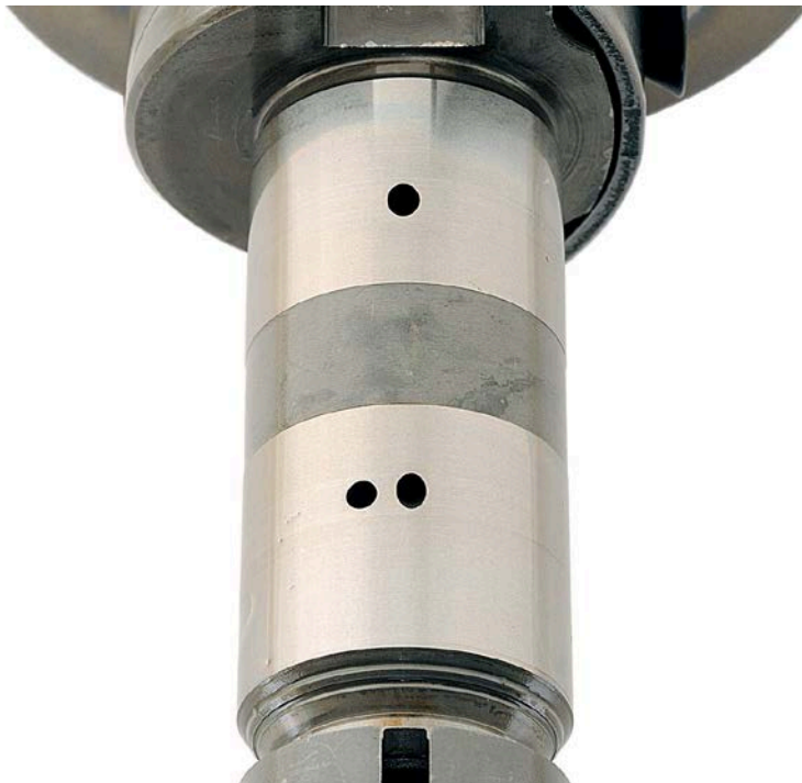
Figure 52. Pump SN:16756536 Distributor Rotor with 1000-Hours Testing with 25/75 ATJ/JP-8 Fuel with 24-ppm CI/LI
