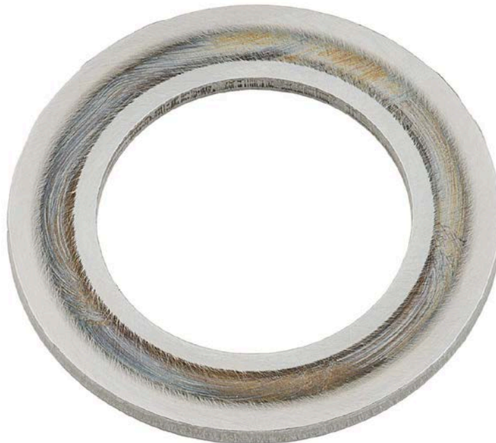
Figure 42. Pump SN:16756535 Thrust Washer with 389-hours Testing with 25/75 ATJ/JP-8 Fuel with 9-ppm CI/LI
