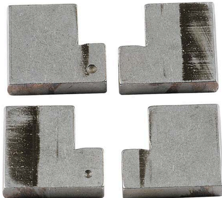
Figure 48. Pump SN:16756535 Transfer Pump Blade Sides with 389-hours Testing with 25/75 ATJ/JP-8 Fuel with 9-ppm CI/LI
