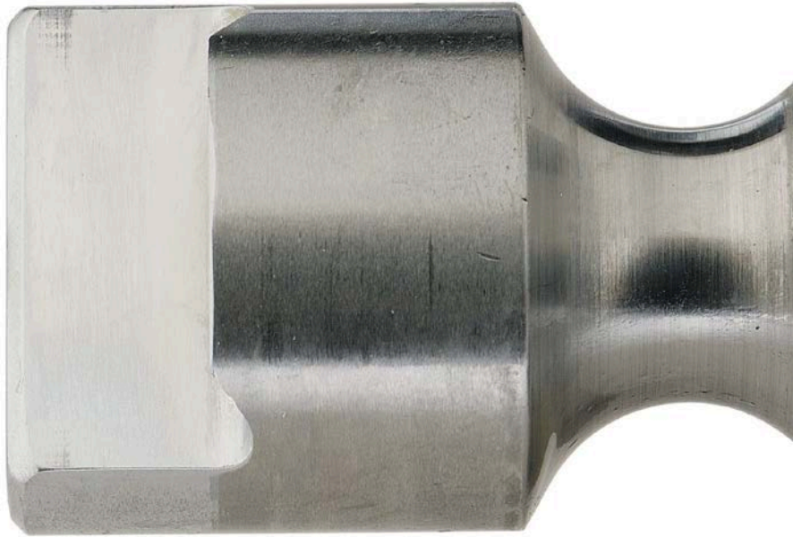
Figure 67. Pump SN:16756536 Driveshaft Drive Tang Sides before Testing with 25/75 ATJ/JP-8 Fuel with 24-ppm CI/LI
