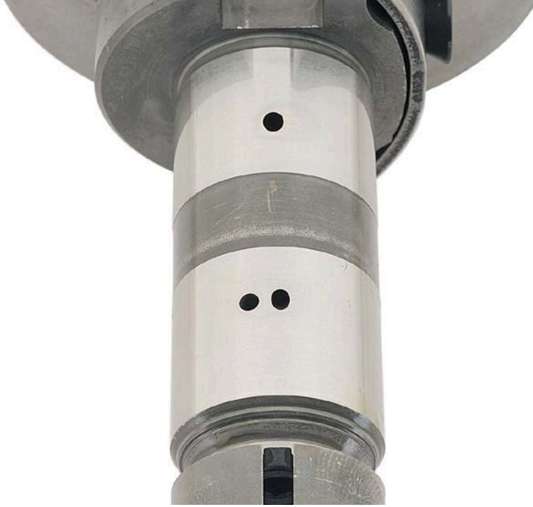
Figure 33. Pump SN:16756535 Distributor Rotor before Testing with 25/75 ATJ/JP-8 Fuel with 9-ppm CI/LI
