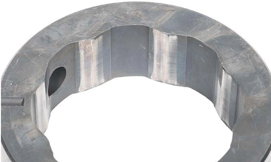
Figure 40. Pump SN:16756535 Cam Ring with 389-hours Testing with 25/75 ATJ/JP-8 Fuel with 9-ppm CI/LI
