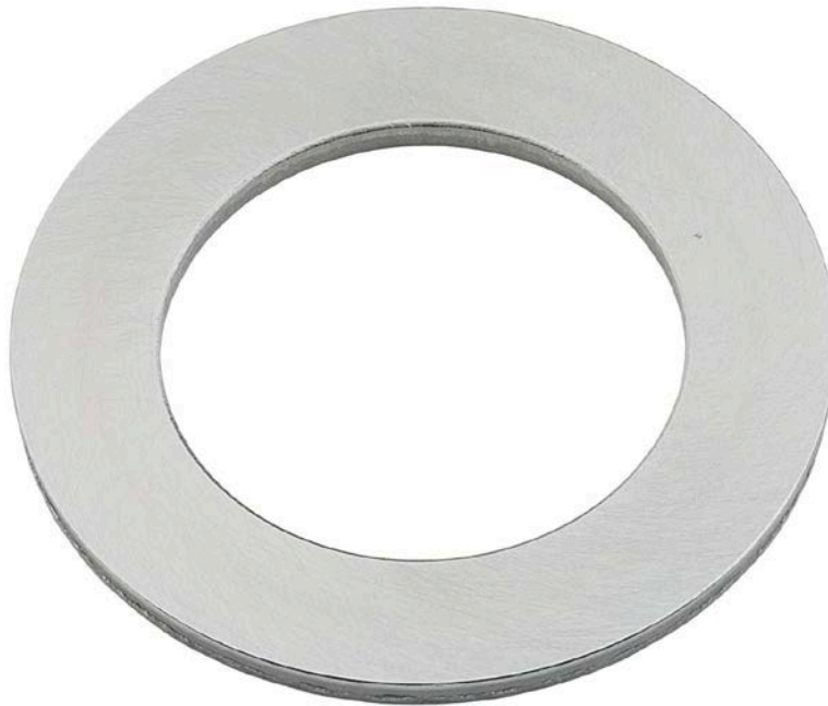
Figure 59. Pump SN:16756536 Thrust Washer before Testing with 25/75 ATJ/JP-8 Fuel with 24-ppm CI/LI
