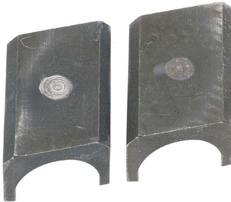
Figure 20. Pump SN:16756534 Roller Shoe with 251-hours Testing with 25/75 ATJ/JP-8 Fuel with 9-ppm CI/LI
