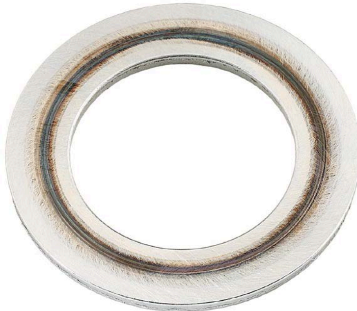
Figure 60. Pump SN:16756536 Thrust Washer with 1000-Hours Testing with 25/75 ATJ/JP-8 Fuel with 24-ppm CI/LI
