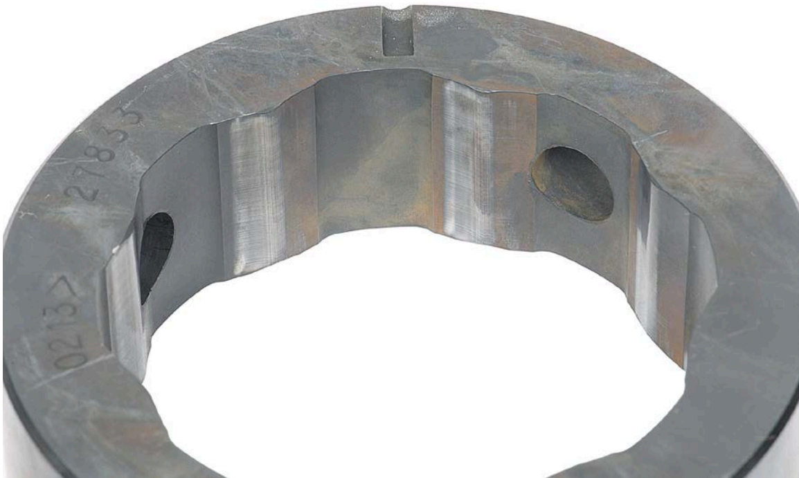
Figure 21. Pump SN:16756534 Cam Ring before Testing with 25/75 ATJ/JP-8 Fuel with 9-ppm CI/LI
