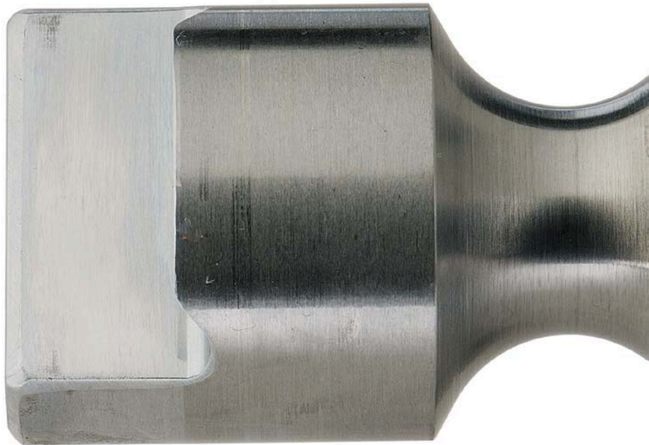
Figure 49. Pump SN:16756535 Driveshaft Drive Tang before Testing
