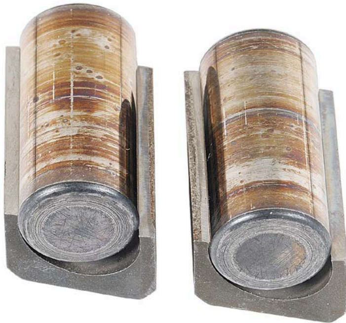
Figure 18. Pump SN:16756534 Rollers and Shoe with 251-hours Testing with 25/75 ATJ/JP-8 Fuel with 9-ppm CI/LI
