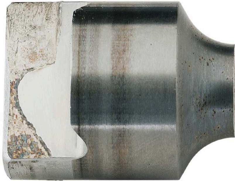
Figure 32. Pump SN:16756534 Driveshaft Drive Tang with 251-hours Testing with 25/75 ATJ/JP-8 Fuel with 9-ppm CI/LI
