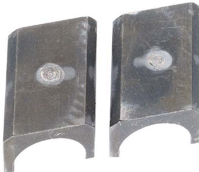
Figure 74. Pump SN:16756538 Roller Shoe with 1000-Hours Testing with 25/75 ATJ/JP-8 Fuel with 24-ppm CI/LI
