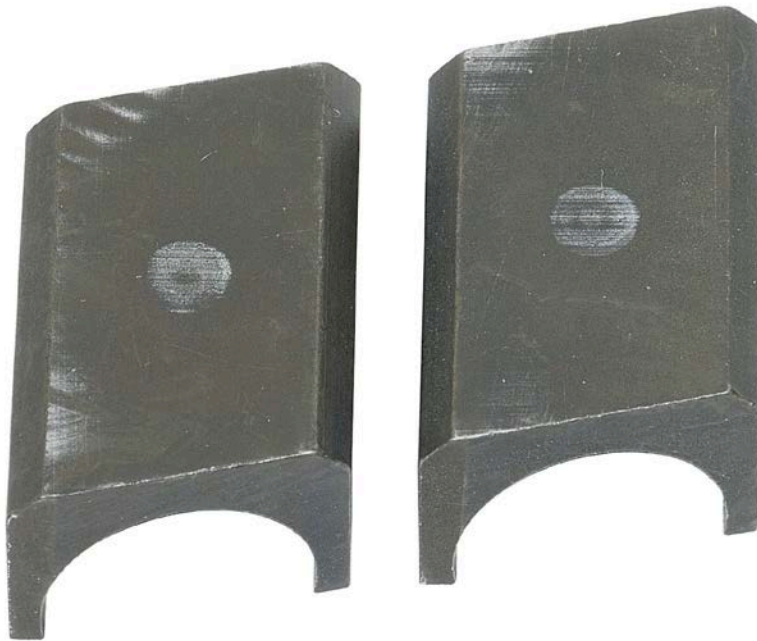
Figure 37. Pump SN:16756535 Roller Shoe Condition before Testing with 25/75 ATJ/JP-8 Fuel with 9-ppm CI/LI
