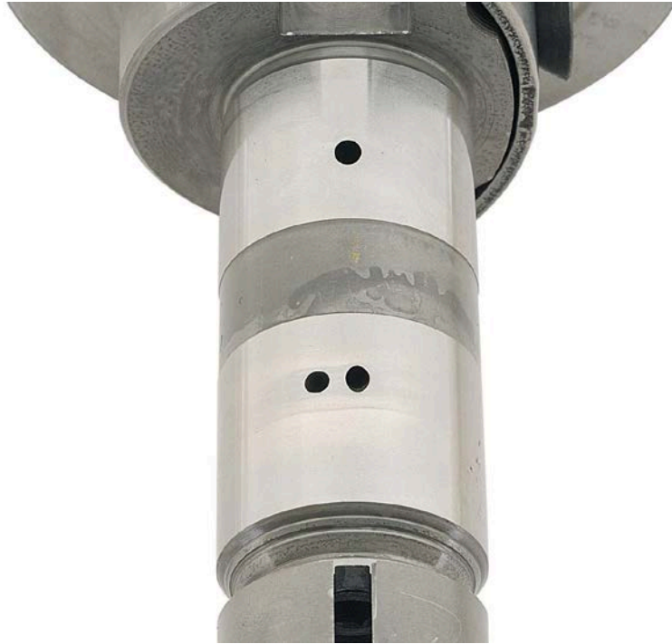
Figure 69. Pump SN:16756538 Distributor Rotor before Testing with 25/75 ATJ/JP-8 Fuel with 24-ppm CI/LI
