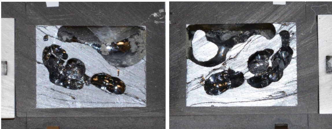
Figure 8.10: Photographs taken after sectioning a test article with a graphite walled PCM cavity. Note the silicon wicked into the upper corners in the front of the test section (center of image) indicating wetting behavior. This is in contrast to the behavior seen in Figure 8.8.
