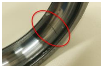
Figure 4: Outer race with a groove shaped fault
