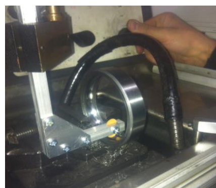
Figure 3: Bearing's outer race in the EDM process
