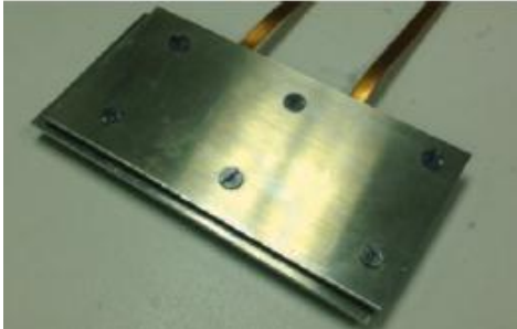
Figure 2. AA7075-T6 and AA2024-T3 lap joint assembly.
