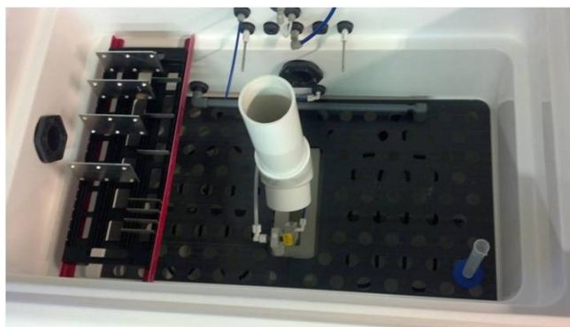
Figure 4. Panels shown in the corrosion chamber prior to the experiment.
