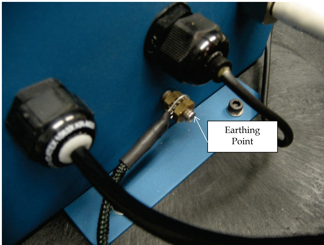
Figure 10: Earthing point on MetalSCAN control box
