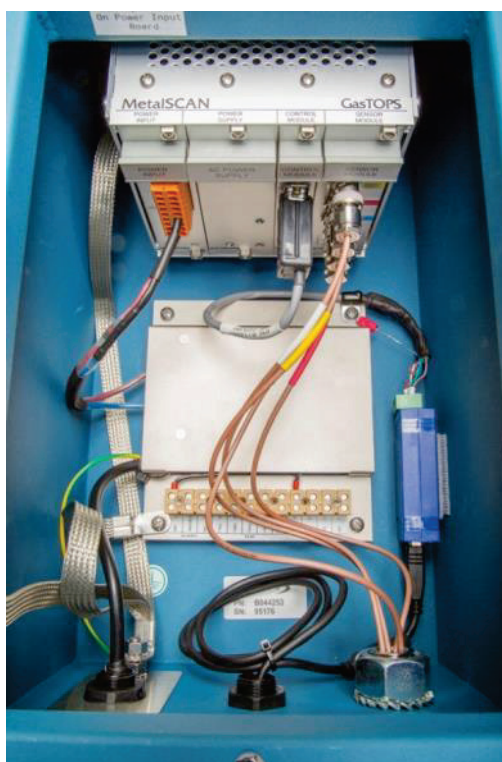
Figure 5: Interior of MetalSCAN control box showing hard-wired modifications
