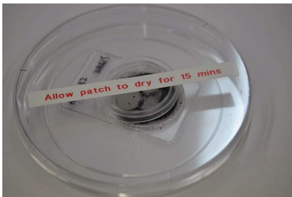
Figure 24: Drying dish with filter patch and petri dish inside
