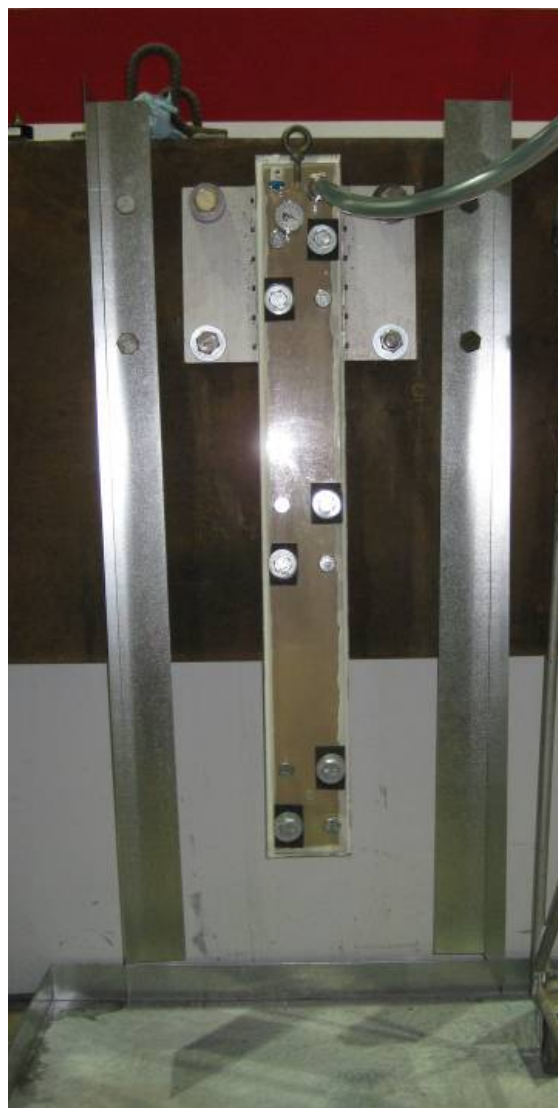
Figure 3-43. Setup for test of silicone caulk on Plexiglas plates.
