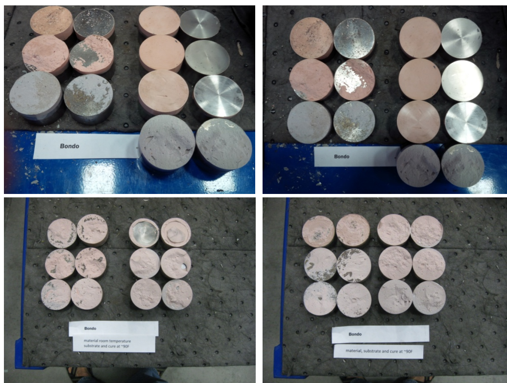
Figure 3-17. Pucks after tensile tests for Bondo®.
