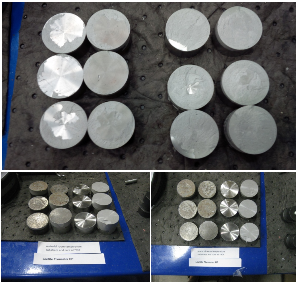
Figure 3-15. Pucks after tensile tests for Loctite Fixmaster® Anchor Bolt Grout HP.
