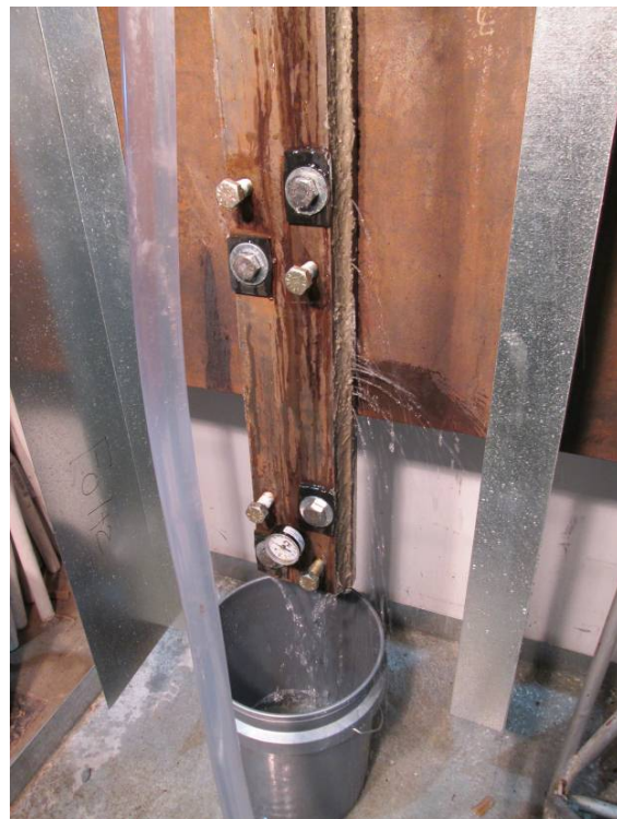
Figure 3-28. Leaks that appeared after applying water pressure to application of Redhead Epcon A7 anchoring adhesive.
