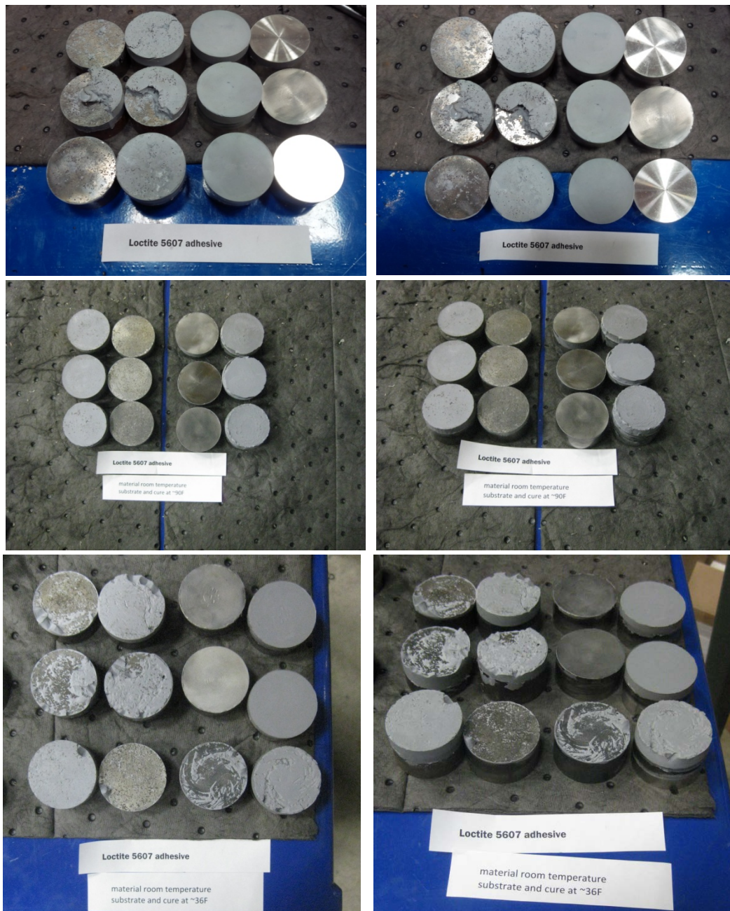
Figure 3-25. Pucks after tensile tests for Loctite 5607 Silicone Adhesive.
