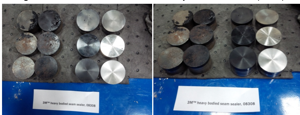
Figure 3-23. Pucks after tensile tests for 3M Heavy Bodied Seam Sealer (08308).
