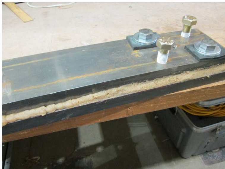
Figure 3-34. Application of Hilti HIT ICE on steel plates at room temperature.
