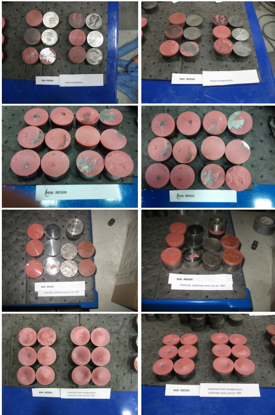
Figure 3-11. Pucks after tensile tests for Hilti HIT RE500.
