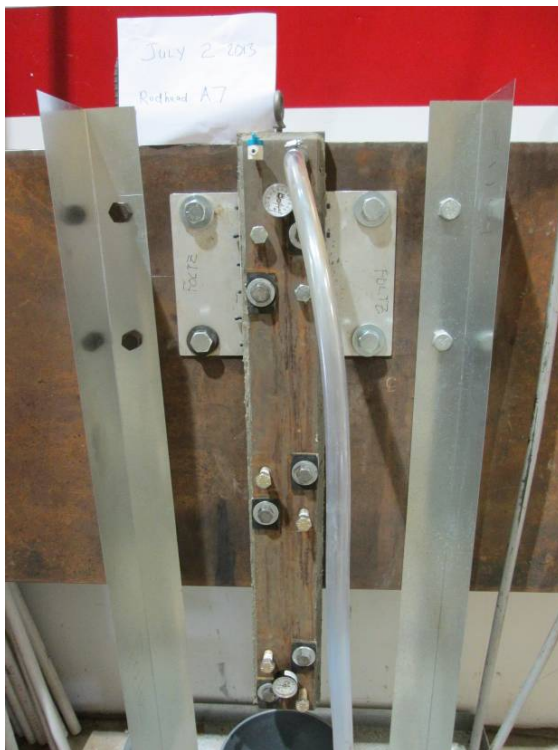
Figure 3-27. Application of Redhead Epcon A7 anchoring adhesive.
