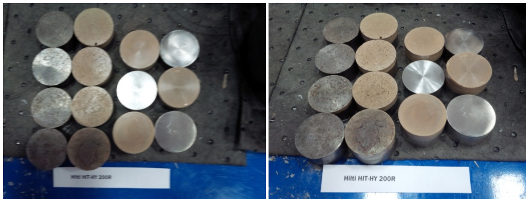
Figure 3-33. Pucks after tensile tests for Hilti HIT-HY 200R / HIT-HY 200A.
