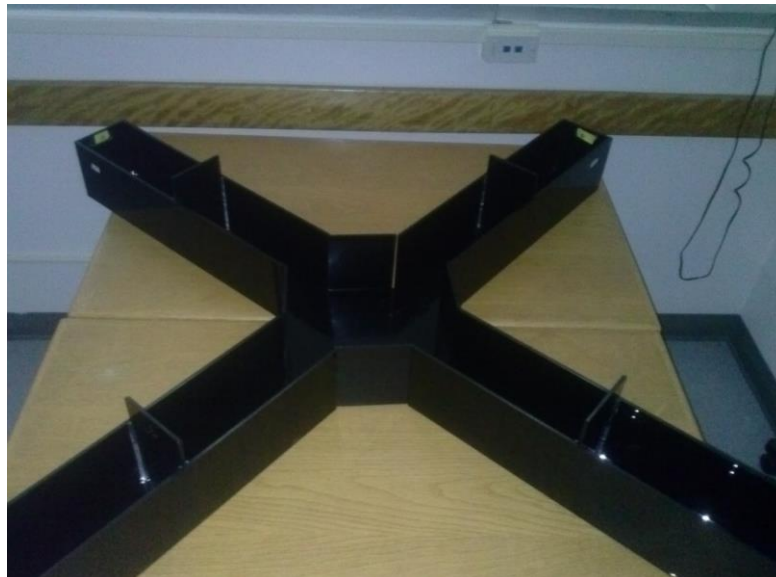
Fig. 6. Image of the maze used for the spatial alternation task. Rats were placed in the middle of the maze and left to explore for 15 minutes. The number and sequence of arm entries were recorded for calculation of a percent alternation score. An alternation consists of 4 different arm choices of 5 consecutive arm entries. A 4/5 percent alternation score was computed by dividing the number of observed alternations in overlapping quintuplets by the number of possible alternations and multiplying the quotient by 100.
