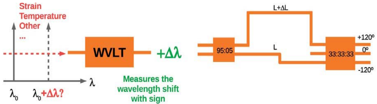
Figure 1. Wavelength tracker concept (a) and sketch of a 2x3 Mach-Zehnder Interferometer based on Multimode Interference couplers (b).
