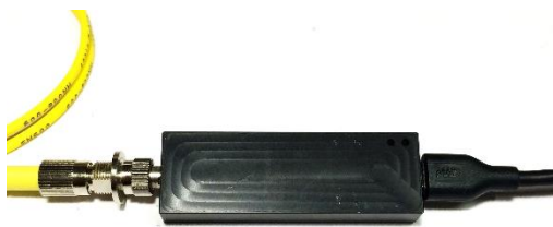
Figure 1 - DPH spectrometer connected to a SM fiber and mini-USB cable
