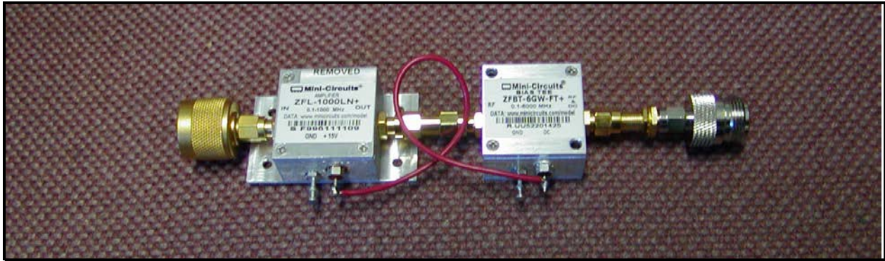
Figure 7. Close-up of the mini circuits ZFL-1000LN+ preamplifier connected to the mini circuits ZFBT-6GW-FT+ bias tee.
