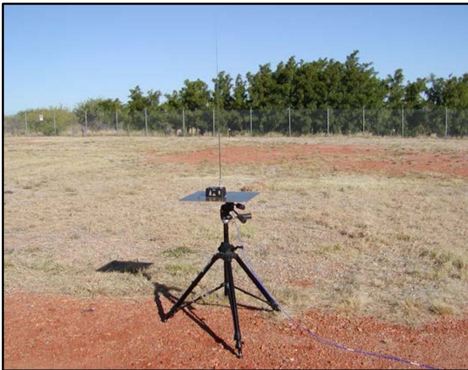
Figure 3. Antenna with rod erected in an open field.
