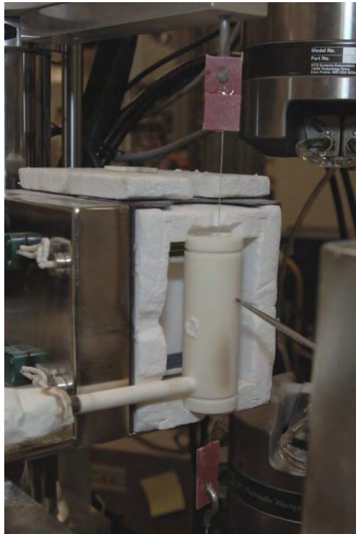
Figure 21. Alumina susceptor and feed tube assembled in one half of the furnace, reproduced from [4]
