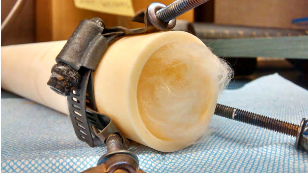
Figure 32. Saturation chamber for silicic acid-saturated steam
