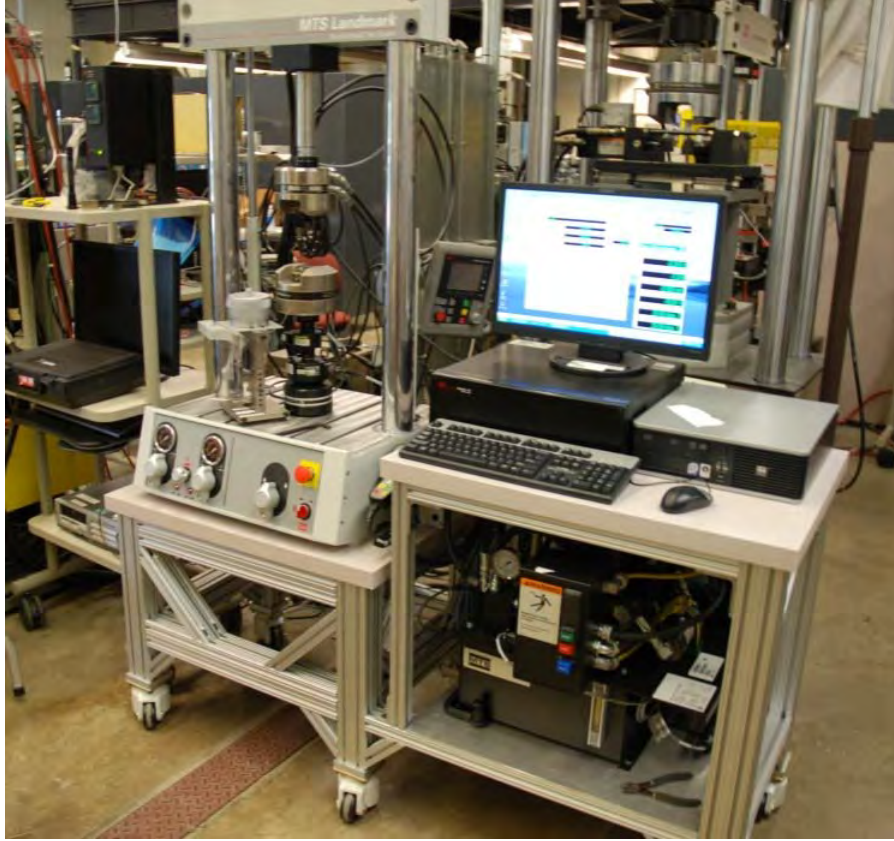
Figure 25. MTS Landmark TM 370.02 servohydraulic test facility, reproduced from [4]
