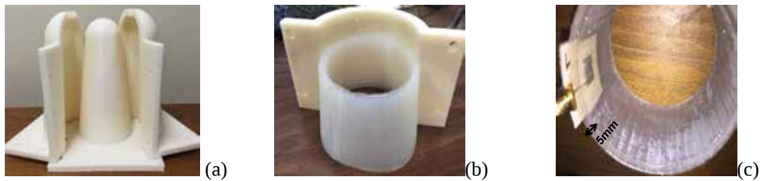
Figure 9: Fabricate shear/ pressure antenna sensor on curved surface; (a) 3D printed casting mold; (b) fabricated custom-made liner by casting method; (c) a patch antenna sensor embedded with the curved surface custom-made liner.
