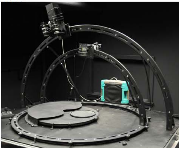
Figure 1. The DRDC goniometer
