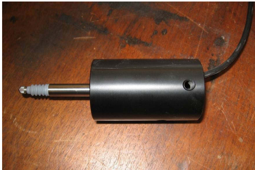
Figure 7: Photograph showing a LVDT transducer installed in a polymer shroud.
