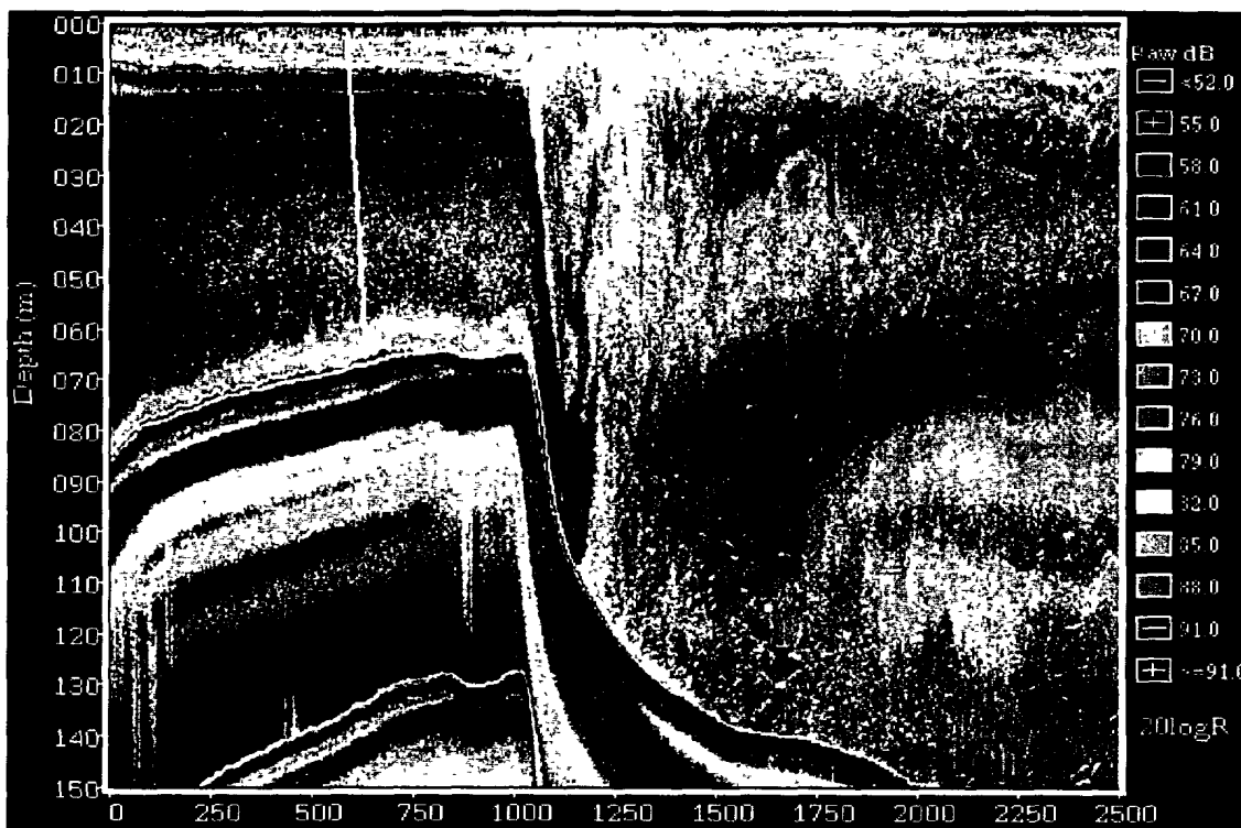
Figure 14 Raw 200 kHz echo-Sounder intensity vs. depth and time (seconds) starting 1514Z Aug. 30 th , 1995 from RV Miller heading from east to west across sill during ebb tide. Tidal flow is from left to right. AMP profile 15770 indicated by white line near time = 600 s.
