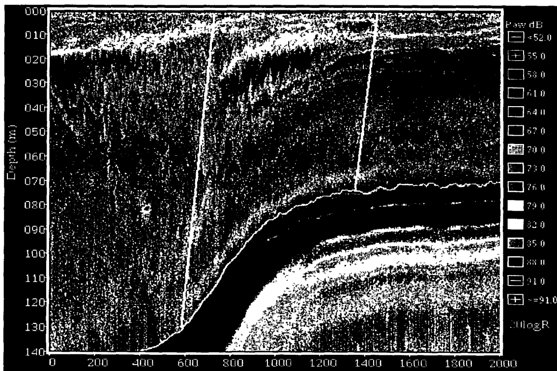
Figure 16 Raw 200 kHz echo-Sounder intensity vs. depth and time (seconds) starting 2232Z Sept. 1 st , from RV Miller heading from east to west across eastern side of sill during flood tide. Tidal flow is from right to left. AMP profiles indicated by lines at 600 and 1400 s.
